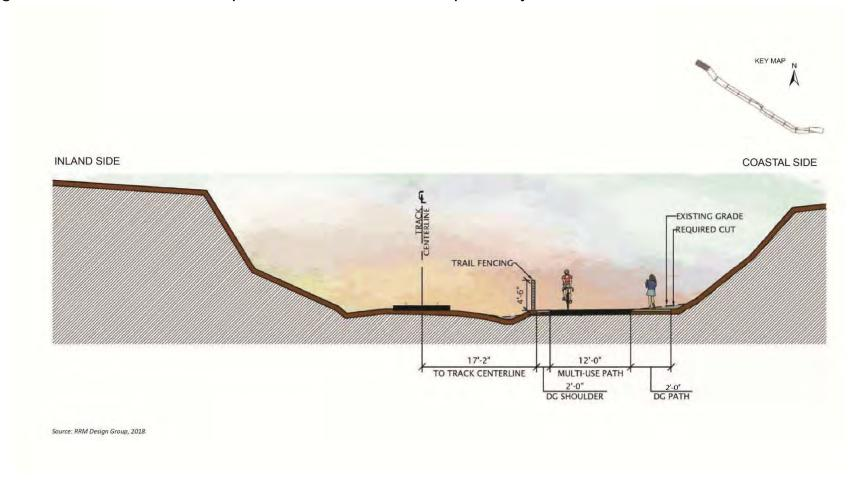
Figure 2-2b North Coast Rail Trail Representative Cross-Section of Proposed Project
