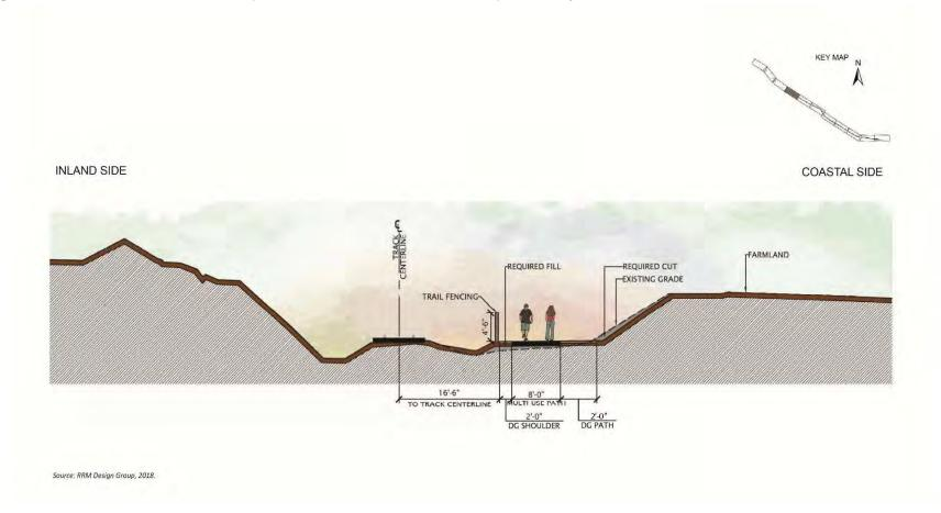
Figure 2-2c North Coast Rail Trail Representative Cross-Section of Proposed Project
