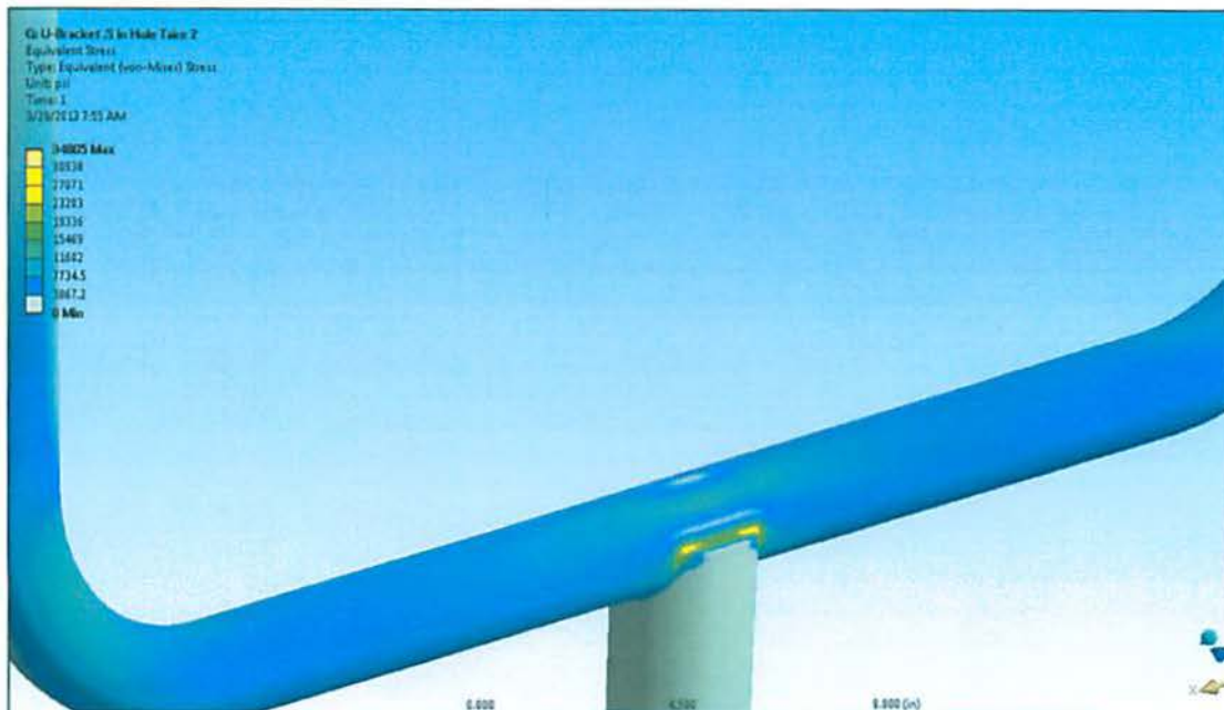
Figure 3 - Result for 1/2" Diameter Drain Hole, Oblique View.
