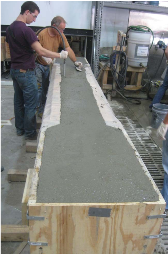
Photo of casting structural element from Purdue University
