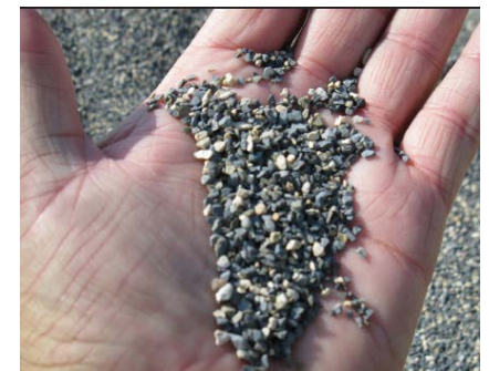
Calcined bauxite provides the long-lasting high friction of HFSTs. (Source: University of Kentucky)
