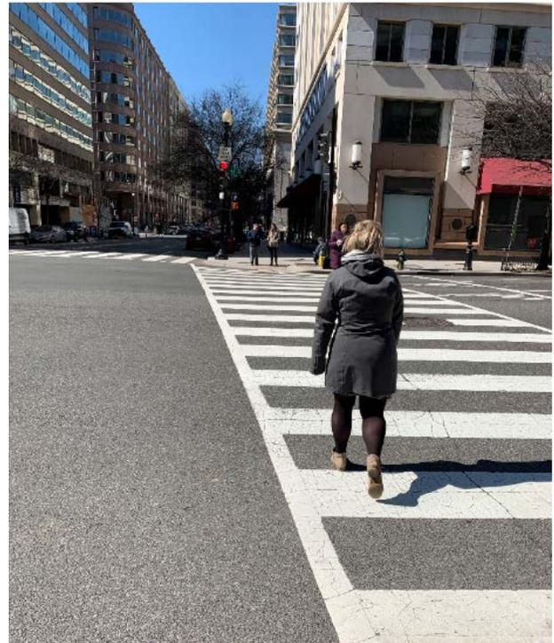
*An LPI allows a pedestrian to establish presence in the crosswalk before vehicles are given a green indication. Source: FHWA.*
