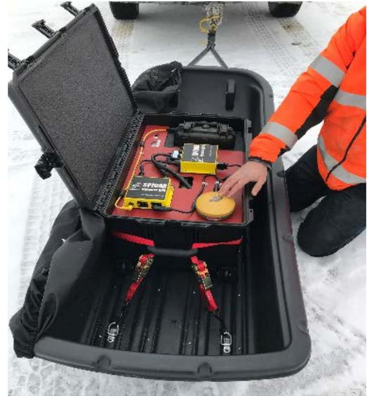
*Ground penetrating radar sled used to monitor ice road thickness.*
