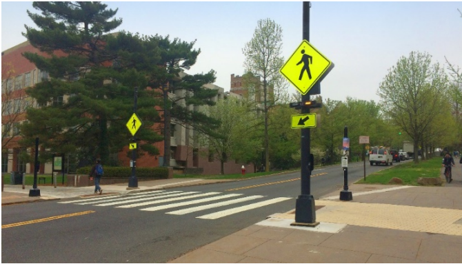
Mid-block pedestrian crossing location with crosswalk visibility enhancements. Photo courtesy of VHB.
