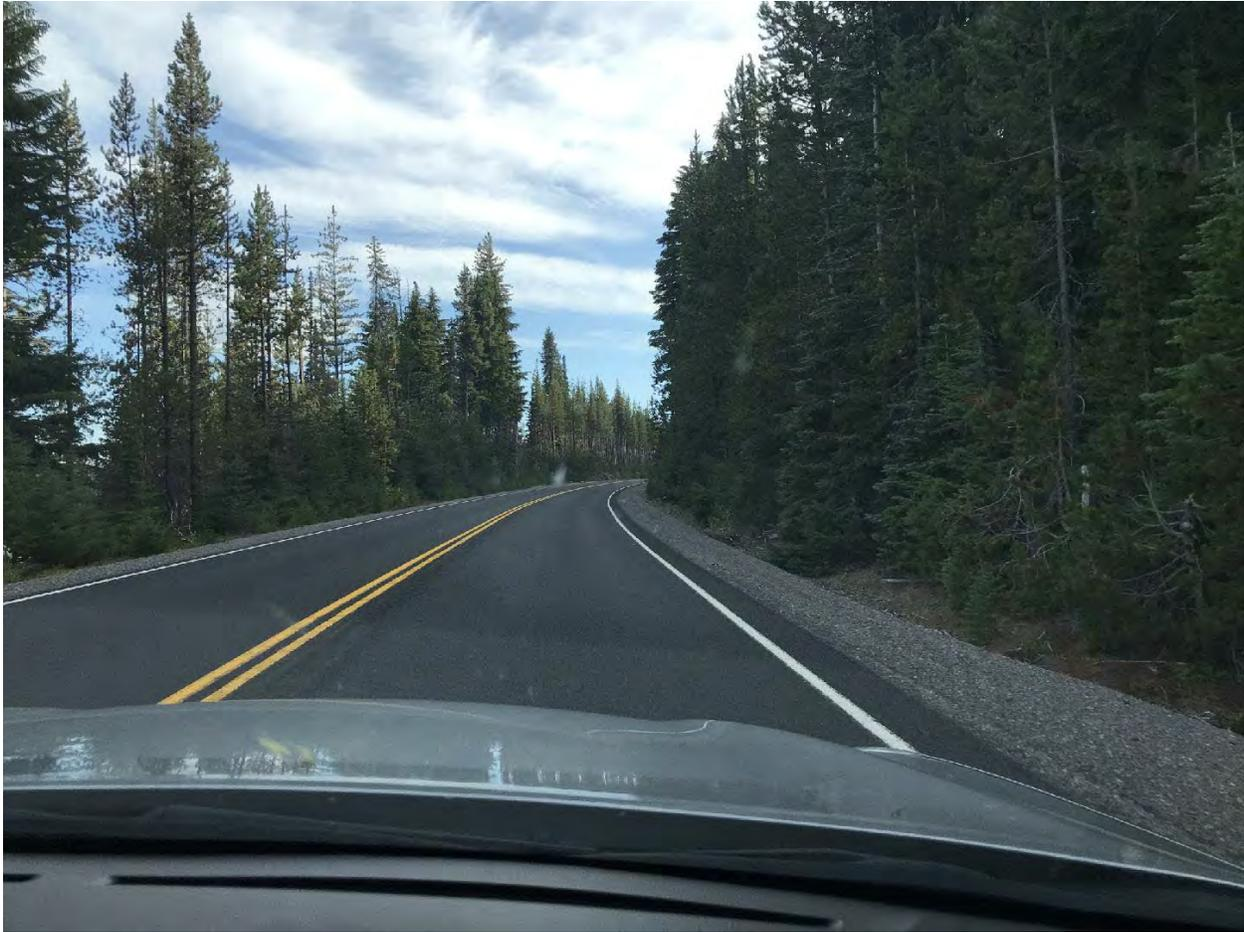
*Figure 15 - Limited Horizontal Sight Distance in Section 6*
