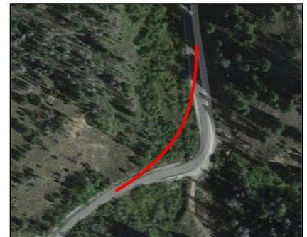
*The 90-degree curve at MP 0.5 would be flattened to achieve a 40-mph design speed.*
