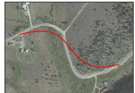
*The horizontal curves on the s-curve section between MP 2.2 and 2.4 would be flattened and a consistent, increasing grade would be established.*
