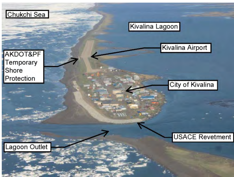
Figure 4: Aerial photo of the City of Kivalina, Kivalina Airport, and previous shoreline protection efforts (Source: WFL).
