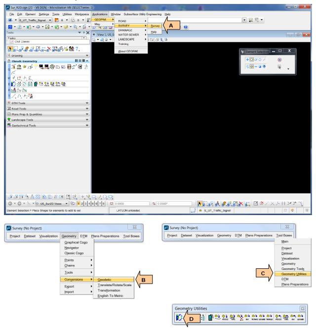
Once the Geodetic Coordinate Conversions tool is activated the user should set the source and target coordinate systems to be able to convert State Plane coordinate values to LAT/LONG.
