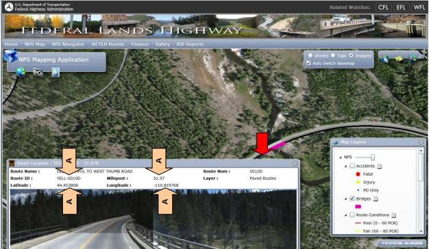
The tool can also be used to get LAT/LONG coordinates even if the route is Unable to be found (for non-NPS Routes – anywhere on the map) LAT/LONG coordinates are displayed for any point clicked by the mouse and these coordinates can also be Copy/Pasted.
