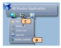
With the Route Location Tool activated click the point on the map, on the route, where the project beginning or ending is located (if a message location not found appears, try the point again), an output window will appear with the Route ID and milepost of the location clicked. Use these values as the EEBACS information. The bottom right corner of the map also tracks the coordinate location of the mouse.
