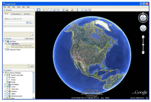
Navigate in Google Earth to the termini location of the project/schedule for the route. Map navigation can most easily be achieved by using the mouse to pan (left-click-press and hold) and using the mouse wheel to adjust the zoom level of the map.
