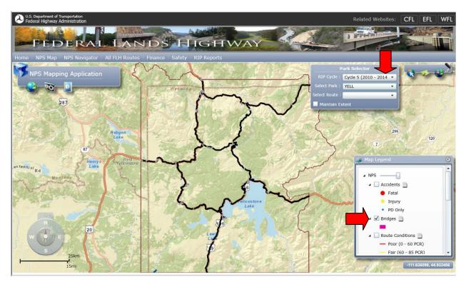
Once the user has navigated to a termini point (beginning or end) of the project by using mouse navigation(mouse wheel for zooming, and point click-hold for panning), other tools are available to query the map to determine the GIS route information for EEBACS.
