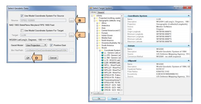
Once the correct Source and Target coordinate systems are set, the user can enter the state plane coordinate values into the tool to calculate the LAT/LONG value for EEBACS. The LAT/LONG value in the tool is shown in Degrees, minutes, and seconds. **This value will need to be converted to decimal degrees.**
