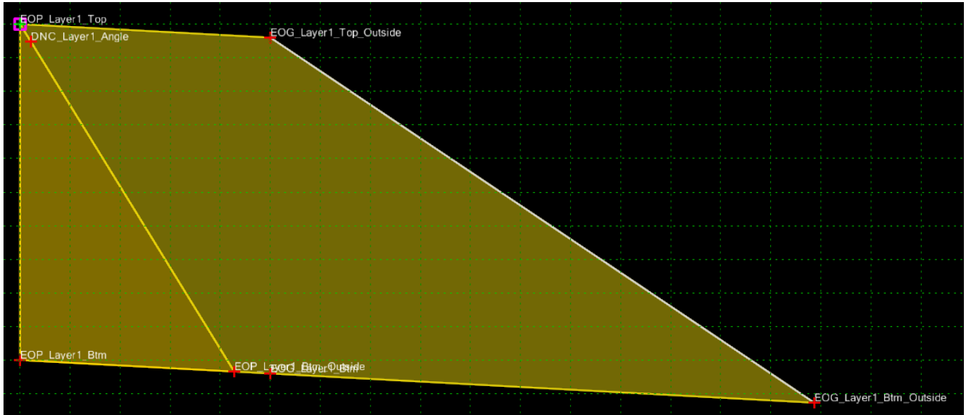
Figure 27 – Safety Wedge Layer 1 Template
