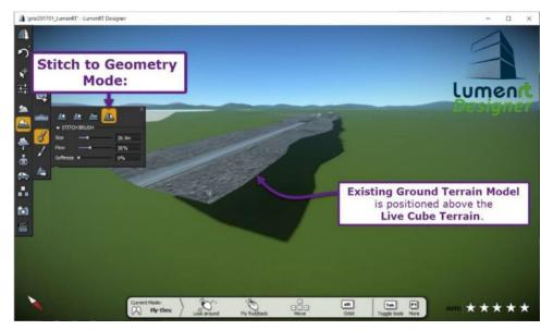
In the workflow shown below, the **Stitch to Geometry** mode is used to raise the LumenRT terrain to meet the perimeter the Existing Ground Terrain Model. In this operation, the User must move the mouse-cursor along the perimeter of the Existing Ground Terrain Model.
