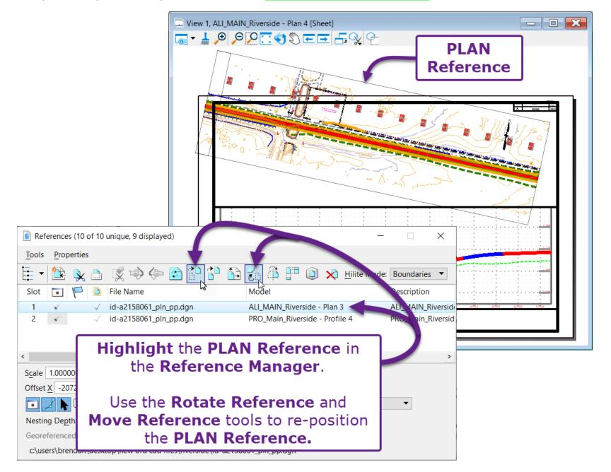
**PROFILE** *Named Boundaries* behave differently than PLAN *Named Boundaries*. The Profile and Existing Ground linework automatically re-positions as expected and the PROFILE *Named Boundaries* remain attached to the original station limits, which are typically even, round values (i.e., STA 13+00 to 15+50).
