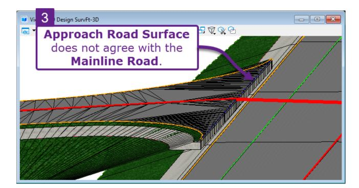
Ensure that horizontal and vertical positions of the edge-of-approach linework aligns with the Mainline. Edit the elevations of the Approach linework as needed to agree with the edited Mainline Corridor.
