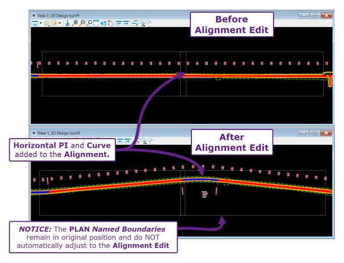
Using the Move and Rotate tools, the PLAN Named Boundary elements can be re-positioned around the edited Alignment.
