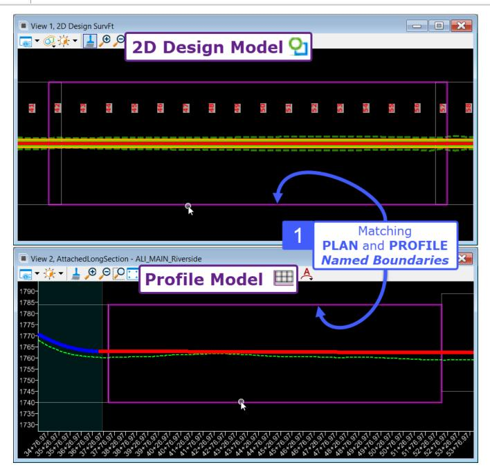
The *Line Between Points* tool (Horizontal ORD Line) can be used to coordinate a location in the *Profile Model*  $\blacksquare$  with a corresponding location along the Alignment in the *2D Design Model*  $\Omega$ . For the "Start Point" of the Horizontal ORD Line, select a location in the *Profile Model*  $\blacksquare$ .
