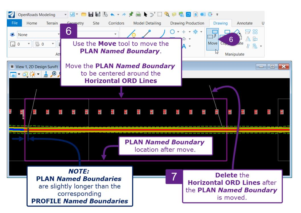
As shown below, there is NO adjustment needed in the corresponding *Sheet Model* because the PLAN *Named Boundary* was ONLY moved and NOT rotated. However, if the PLAN *Named Boundary* is **rotated**, then the PLAN reference must be manually rotated and moved to realign with the Sheet Border. Moving and Rotating is shown in detail in **14E.1** Rotate and Move Plan Views.
