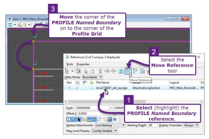
**IMPORTANT:** After moving the PROFILE *Named Boundary* reference, the Profile Grid must be deleted (*Remove Drawing Model Annotations* tool) and re-created (*Annotate Drawing Model* tool). See <u>14E.4.a</u> *Remove Model Annotations tool* and <u>14E.4.b Annotate Model tool</u>.
