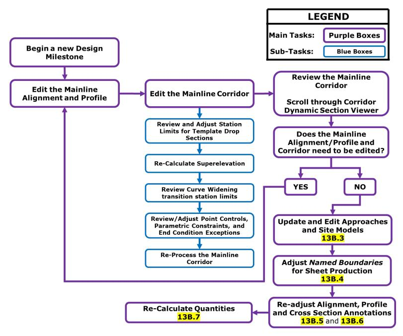
**IMPORTANT:** Edits to the Alignment, Profile, and Corridor affects ancillary modeling features and *Sheet Models Models* . See <u>13A.6 Effects of Modeling Iterations</u> and <u>13B.3 Affects to Named Boundaries and Plan Sheets</u>.
