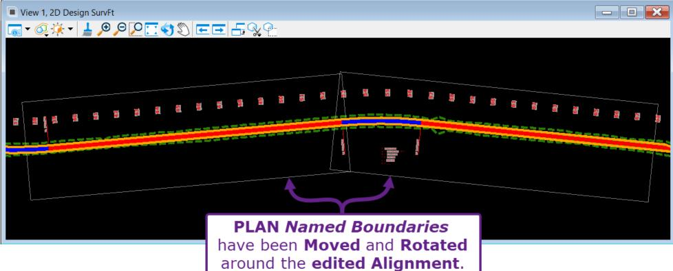
As shown below, after **rotating** a PLAN *Named Boundary*, the PLAN reference in the *Sheet Model* becomes unoriented with the Sheet Border. This is rectified by rotating and moving the PLAN reference with the *Rotate Reference* and *Move Reference* tools found in the Reference Manager. Moving and Rotating is shown in detail in 14E.1 Rotate and Move Plan Views.
