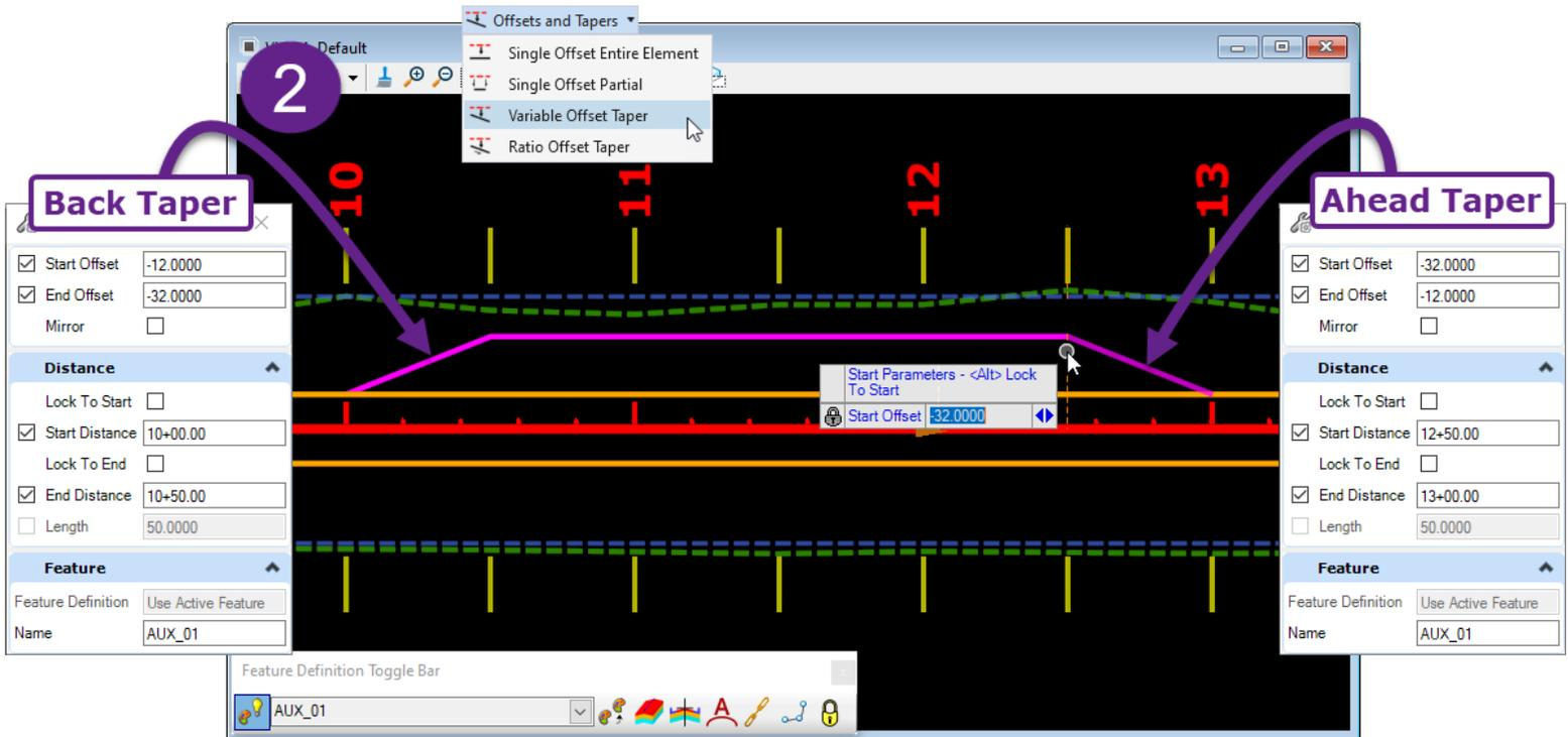
**Create the Point Control geometry:** Using the *Variable Offset Partial* tool, create the back and ahead tapers for the turnout.
