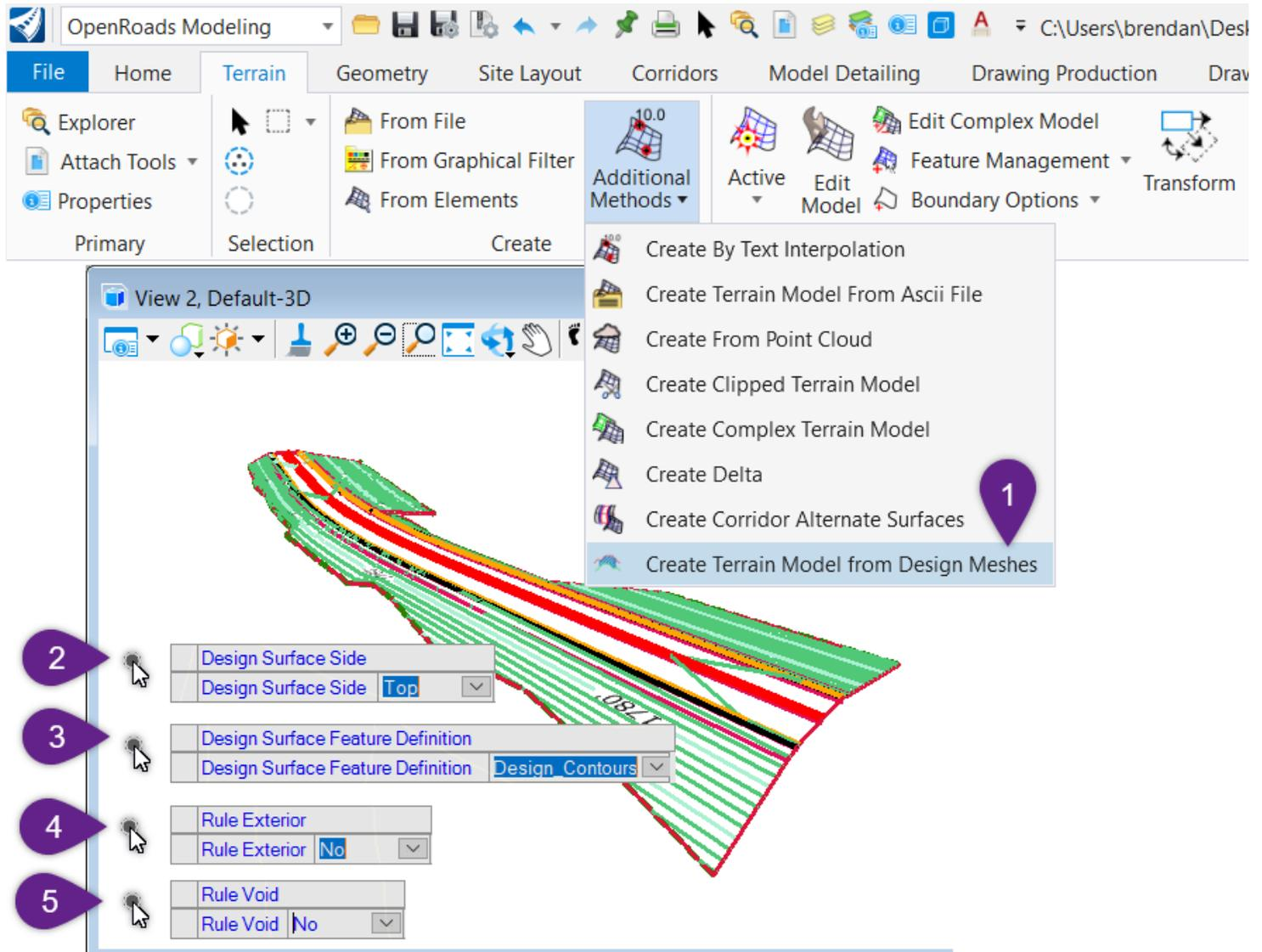
**NOTE:** When this tool is used, a Terrain Model is created for every Corridor, Linear Template, and Surface Template contained in the ORD File. This tool does NOT allow the User to select an individual Corridor.
