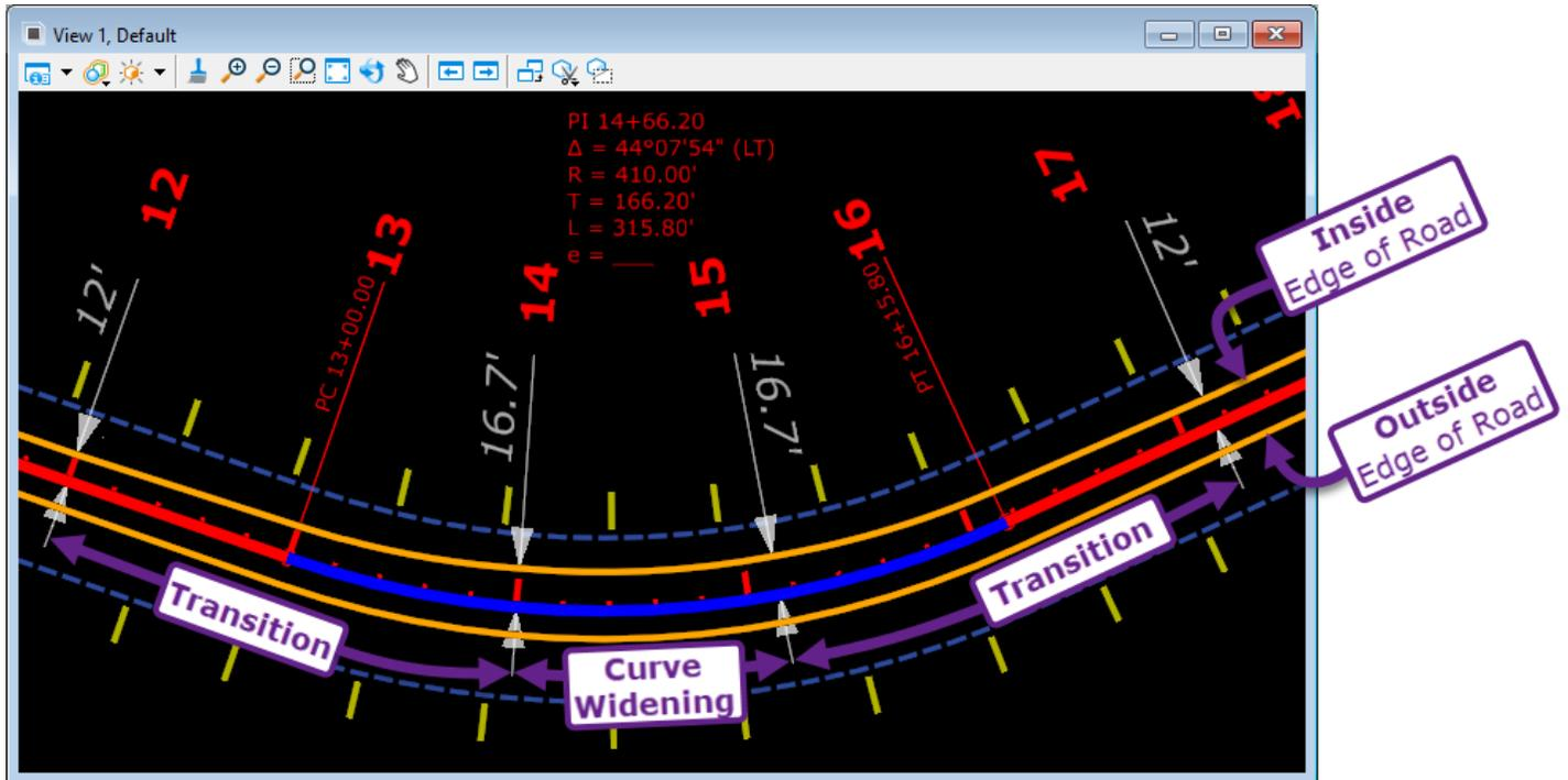
The Curve Widening tool works in conjunction with an external text file which contains a ".wid" file extension type and is referred to as the Curve Widening File. The Curve Widening File contains a simple Curve Widening Table which determines the additional width to be added to a curve and the length needed for transitions.
