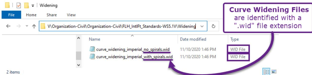
**WARNING:** Do NOT directly edit or use the Curve Widening Files stored on the FLH WorkSpace. Instead, copy the appropriate Curve Widening File from the FLH WorkSpace to appropriate project file folder.
