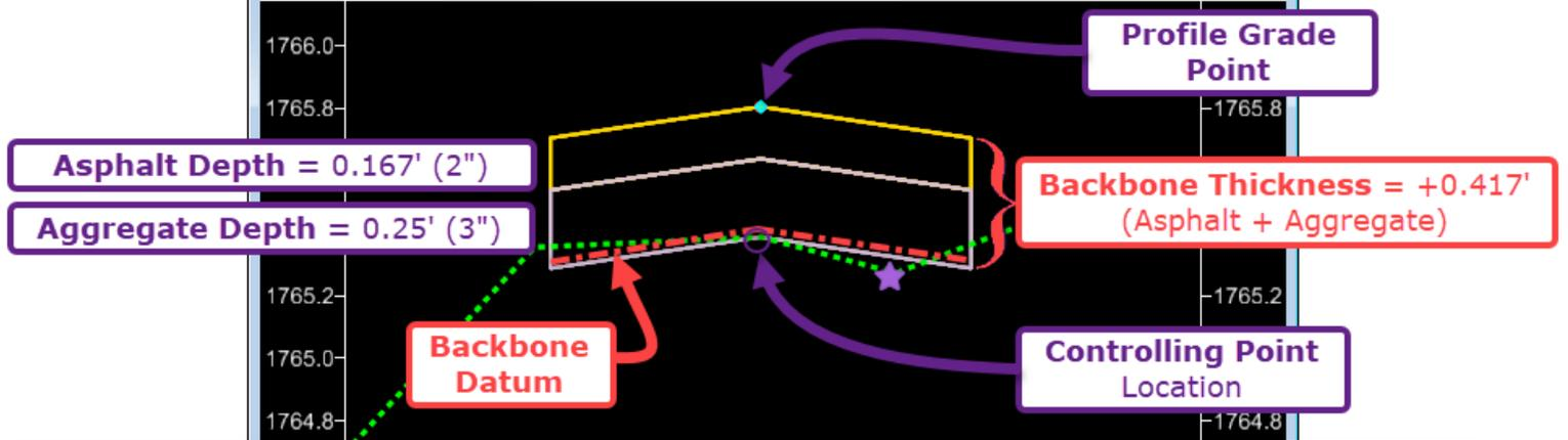
Using the **Minimum Milling** mode, the **lowest** Existing Ground point is selected as the **Controlling Point** location. The **Backbone Datum** is placed directly atop of the **Controlling Point**.
