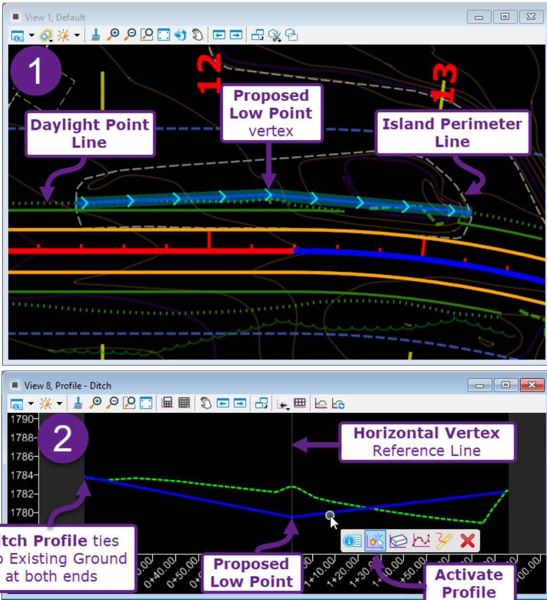
**Create the Point Control Geometry for the Ditch Alignment and Profile Elements:**
