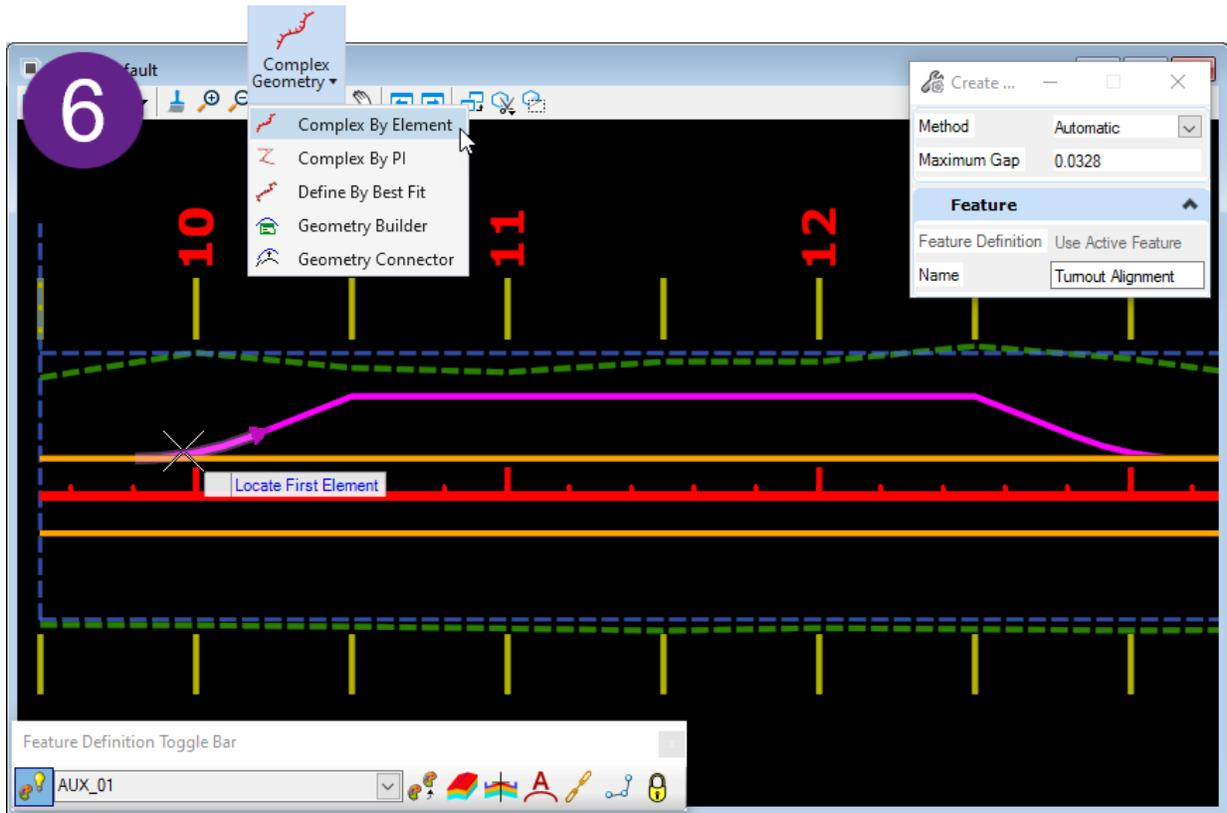
**Create the Point Control Geometry:** Using the *Complex By Element* tool, combine all elements created thus far into a single Point Control alignment.
