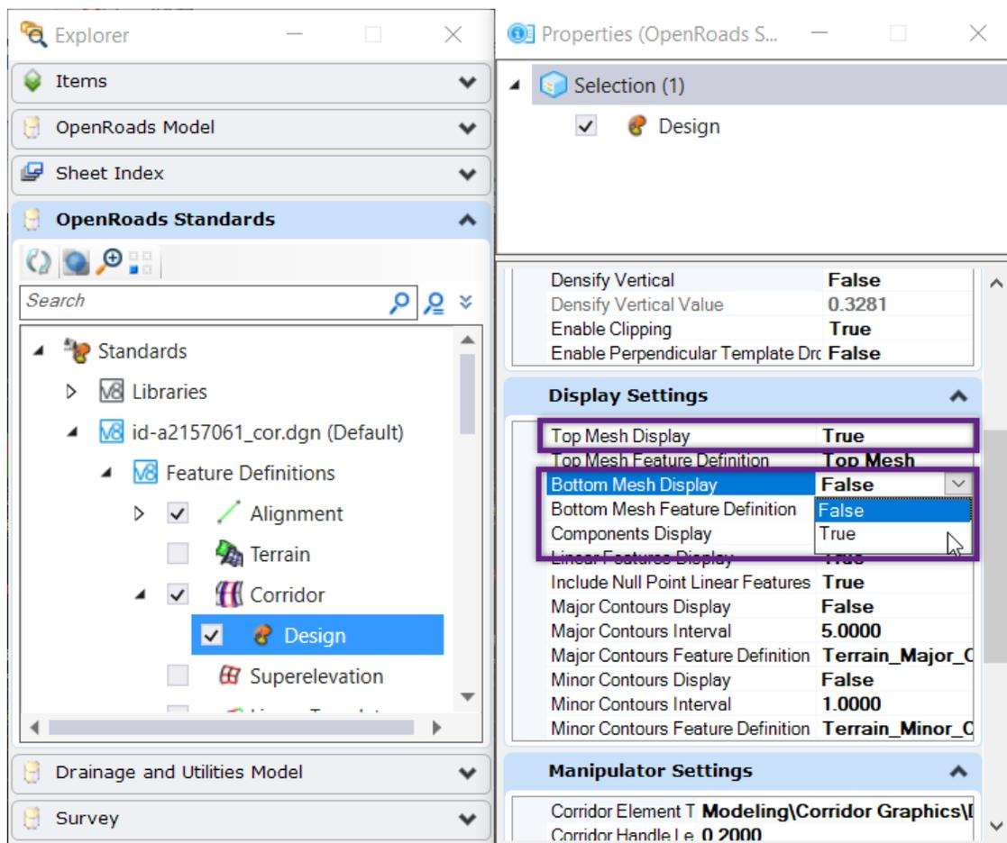
After Corridor Feature Definition display settings are edited, the Corridor must be reprocessed for the Top and Bottom Mesh to finally be displayed.
