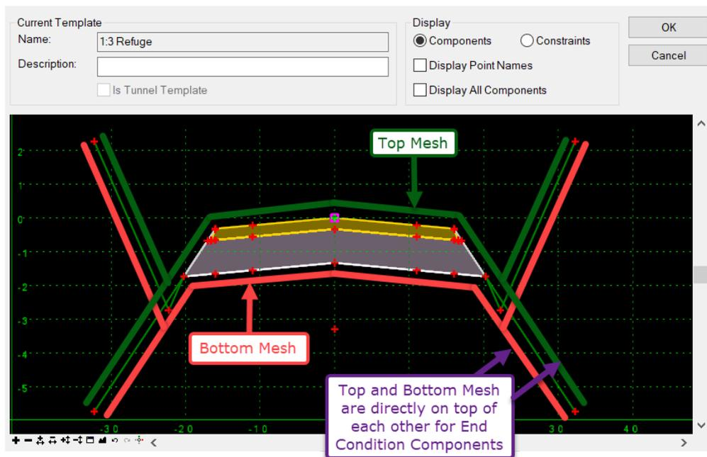
**NOTE:** Mesh Elements are found in the 3D Design Model
