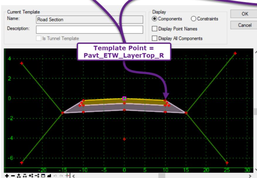
In the demonstration shown above, the pavement width changes abruptly from 10' to 15. It would be practical to create two additional Parametric Constraints to model the back and ahead tapers. Tapering sections are created by varying the Parametric Constraint *Start* and *Stop Values*.
