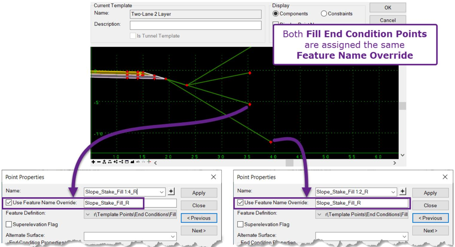
If Fill End Condition points did NOT have identical Feature Name Overrides, then a gap would form where the fill slope transitions from 1V:2H to 1V:4H or vice versa. In the graphic shown below, the **Feature Name Override** boxes are UNCHECKED and disabled.
