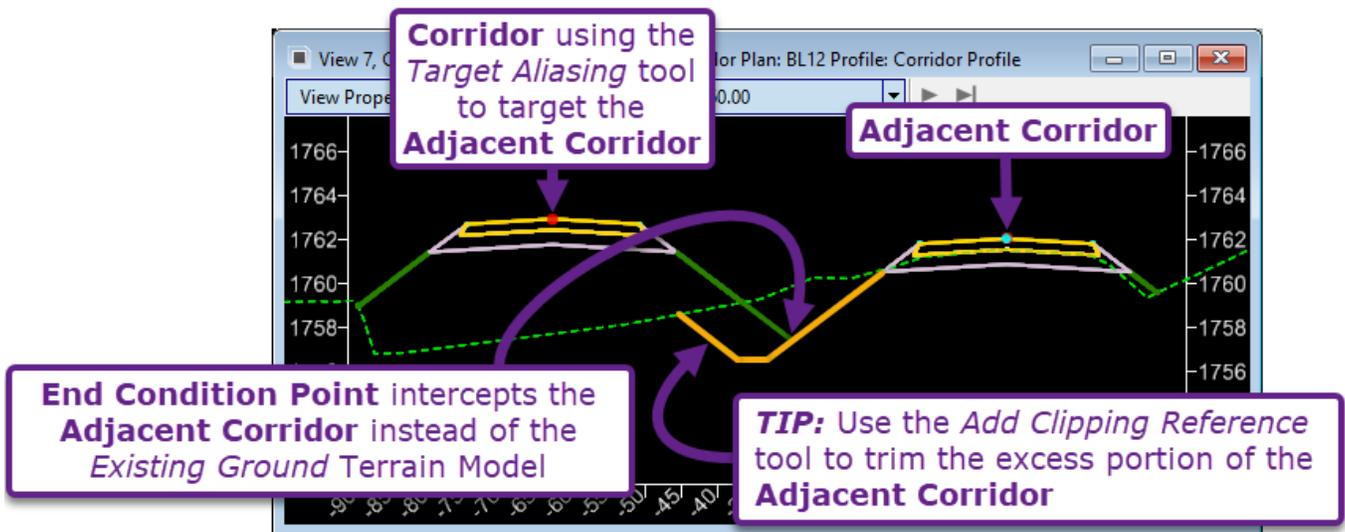
The *Target Aliasing Menu* is used to specify and prioritize Targets that a Corridor will attempt to intercept. When it is possible to solve for more than one target, then the order of the Aliases List (found in the Target Aliasing Menu) determines which target is used.
