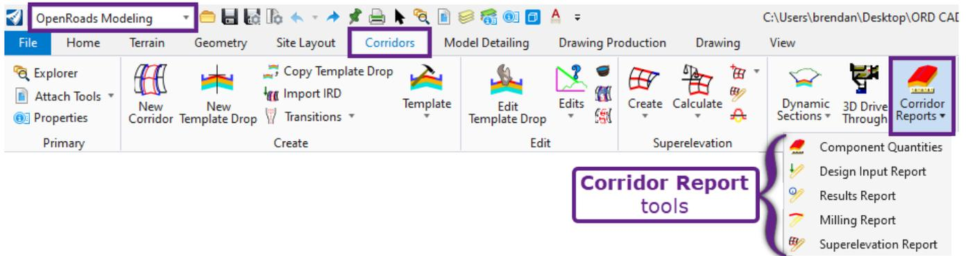
In general, most of the reports are rarely used, except for the **Components Quantities** report. This report can be used to quickly check quantities for a **single** Corridor. The process of calculating quantities for multiple Corridors or a combination of Corridors, Linear Templates, and Surface Templates is discussed in [Chapter 20 – Quantities](#).
