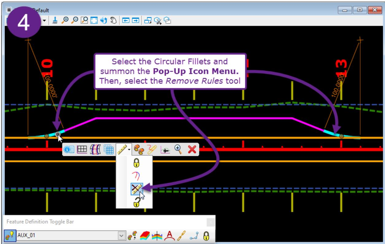
**4 Create the Point Control Geometry:** Use the *Remove Rules* tool to remove the *Dependencies* from the Circular Fillets.
