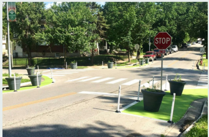
Figure 2. Example traffic calming improvements as part of the Vision Zero program. Source: Kansas City Vision Zero Plan; Street Smarts Design & Build.
