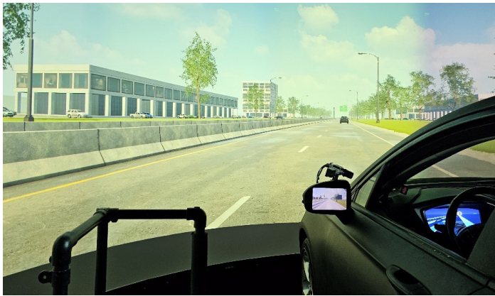
Source: FHWA. The TFHRC highway driving simulator's new visual system features a 220-degree field of view.
