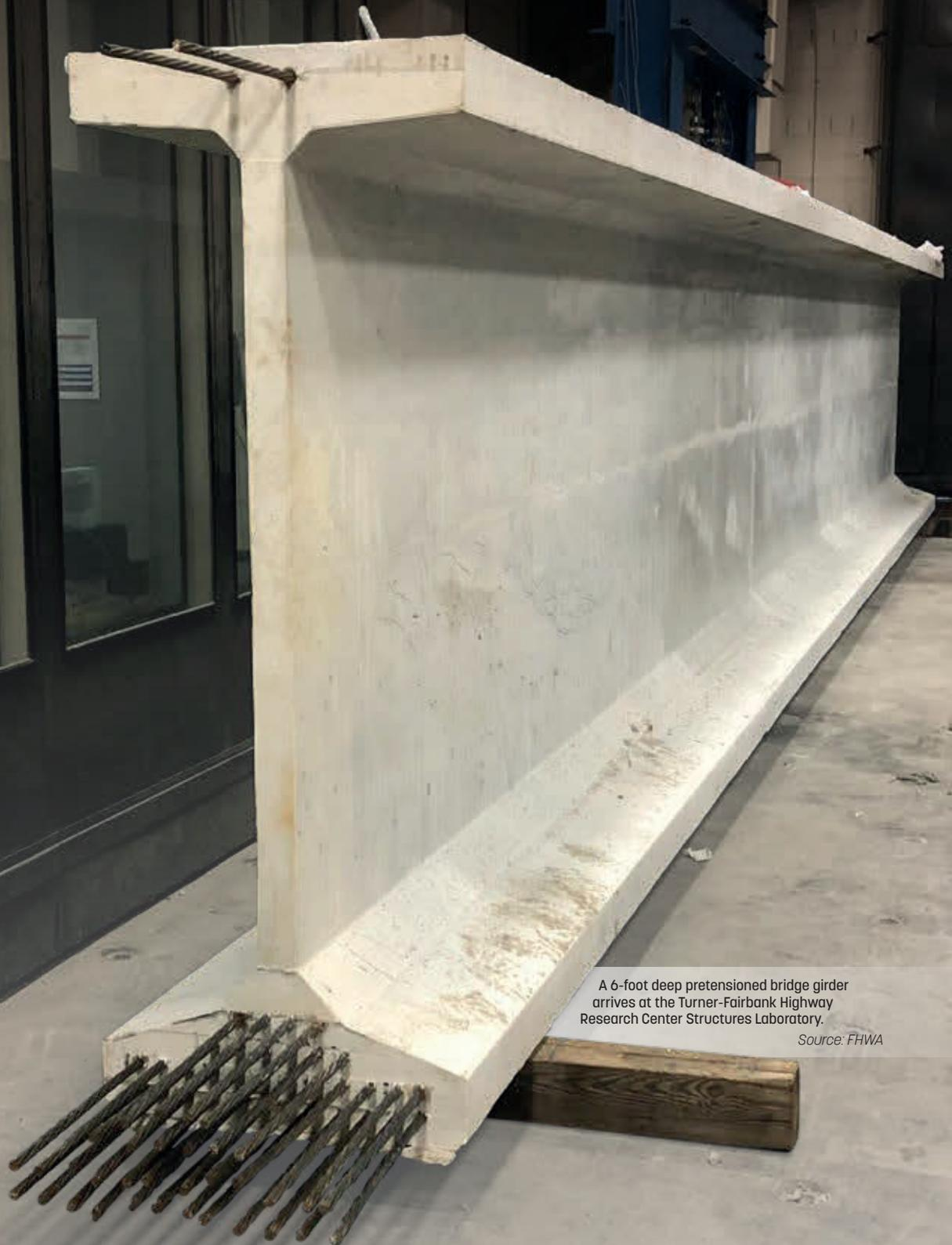
A 6-foot deep pretensioned bridge girder arrives at the Turner-Fairbank Highway Research Center Structures Laboratory.
