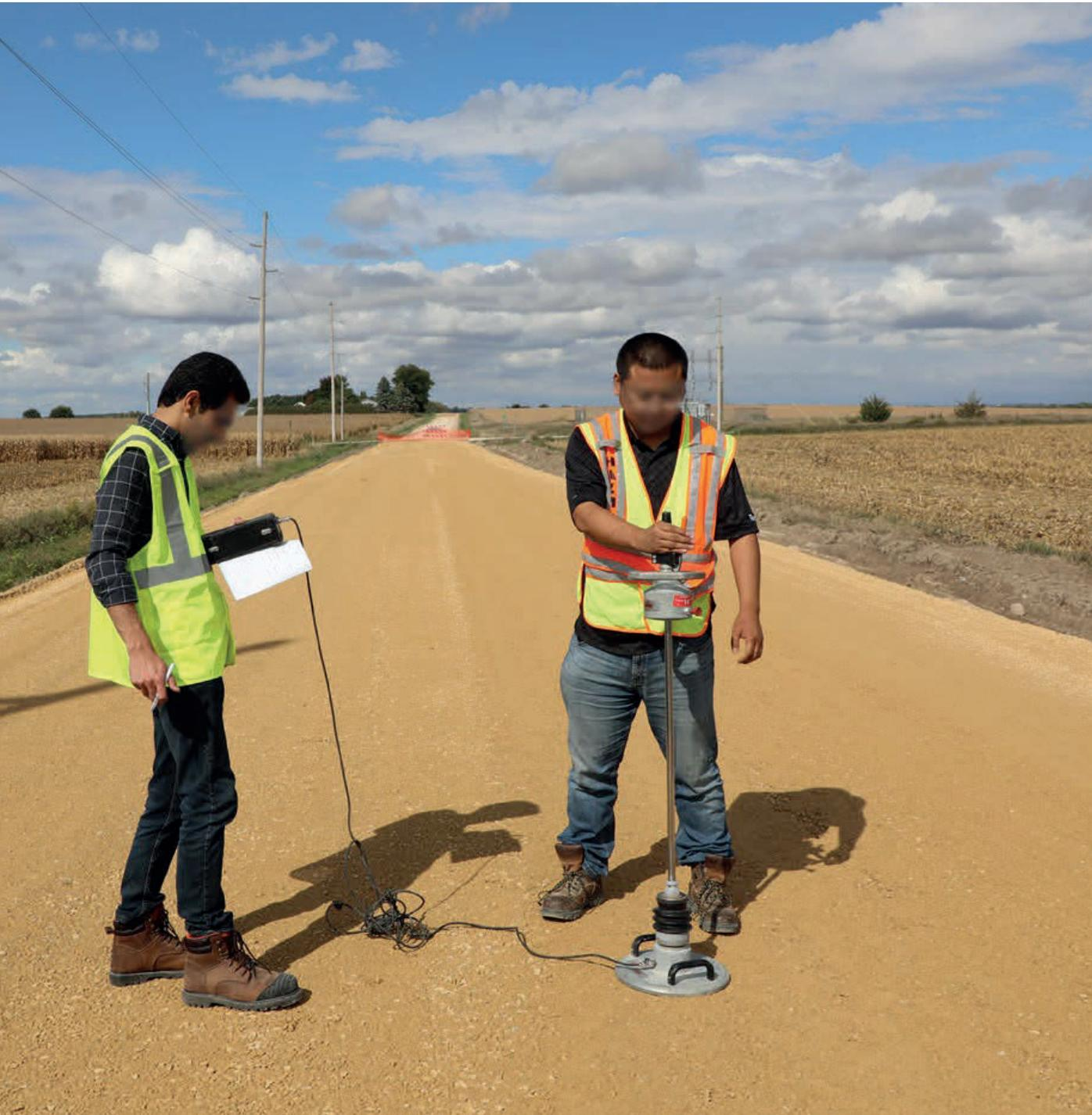
Unpaved road monitoring by field tests (dynamic cone penetrometer test on the subgrade) in Buchanan County.
