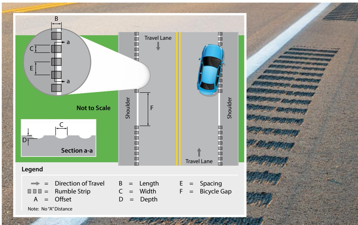
Edge line rumble strips can be directly placed on the shoulder (or bicycle lane) to alert drivers when they are drifting out of their lane.
