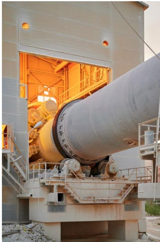
**LEFT:** A giant rotating furnace is used in the factory for roasting limestone.
