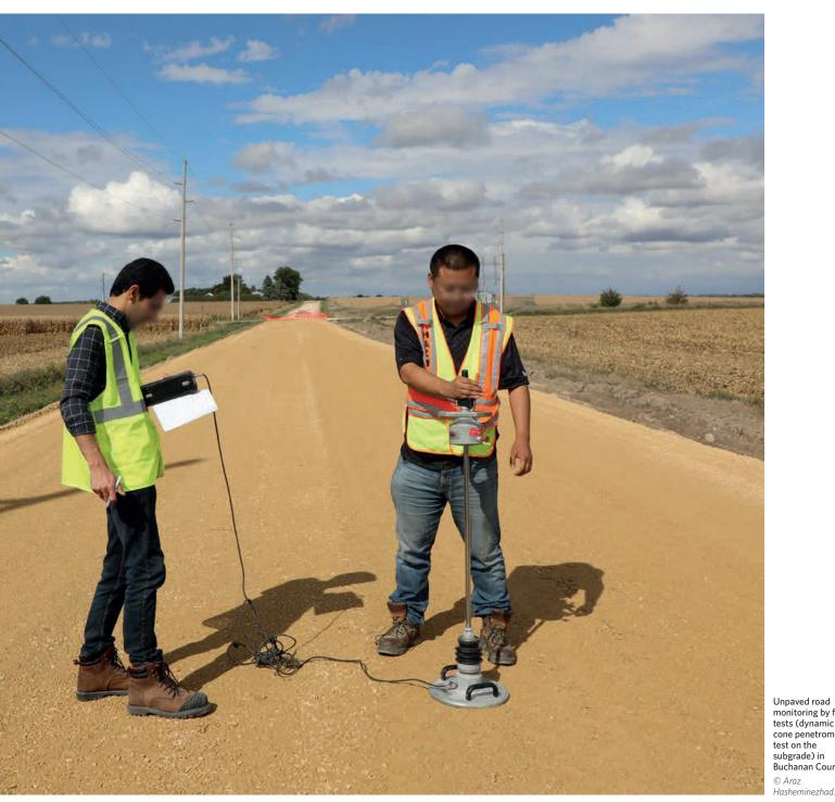
Unpaved road monitoring by field tests (dynamic cone penetrometer test on the subgrade) in Buchanan County. © Araz
