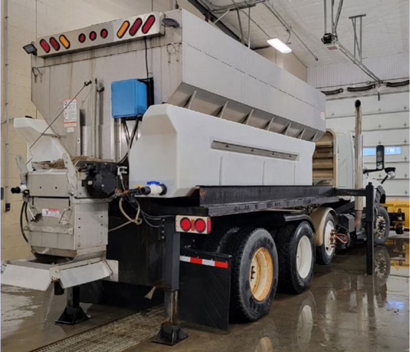
The SMART Transformation Award-winning innovation called the Fifth-Wheel Quick Attach Sander. © 2024 McKenzie County, ND.
