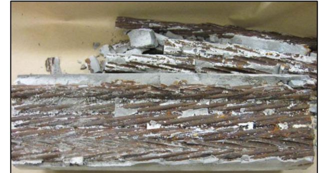
208 days in 5% NaCl fog chamber
