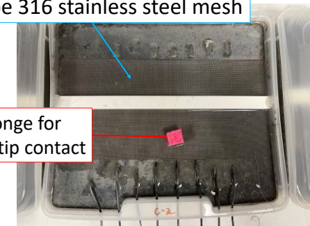
Testing in good-quality grout.
