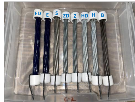
Testing in good-quality grout.
