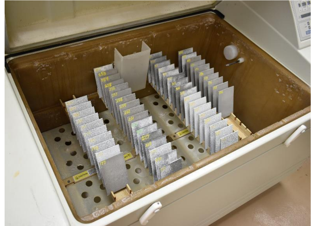
Panels in salt-fog chamber.
