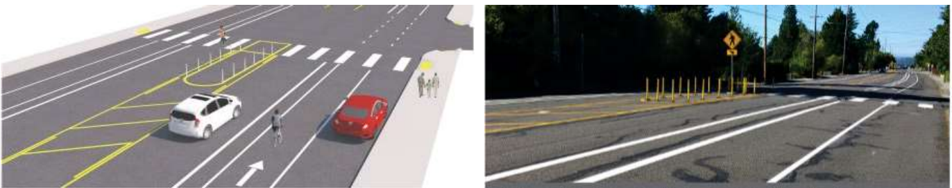
Figure 12. Example of road configuration in Portland after street redesign from five lanes to three lanes.
