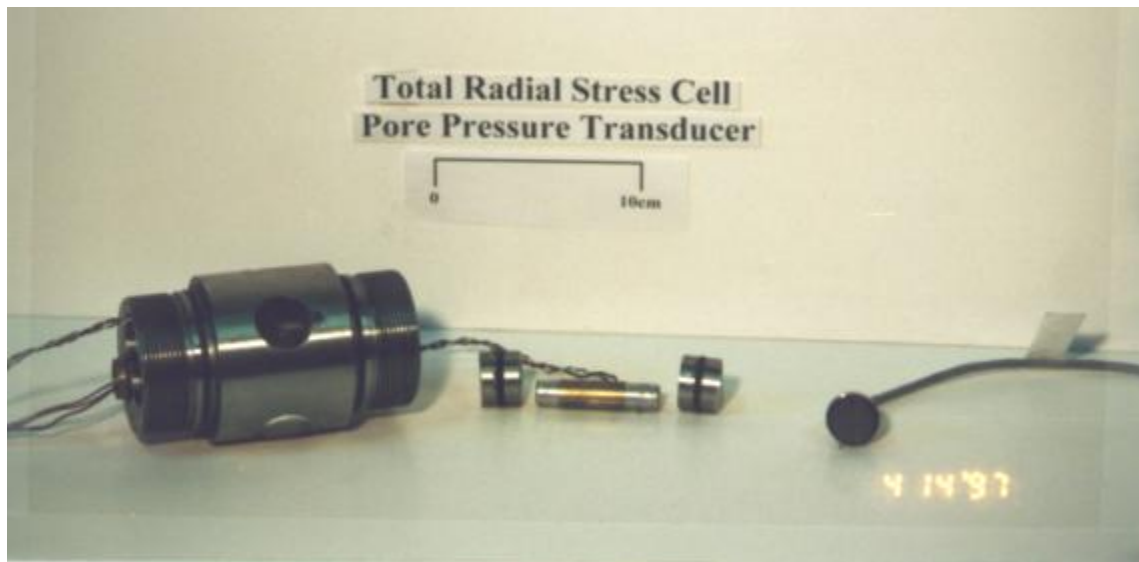
Figure 23. Photograph of the Transducer Housing With the Pore Pressure Transducer and the Total Radial Stress Cell.
