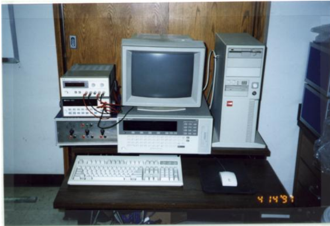
Figure 29. Hewlett Packard Data Acquisition System (HP DAS).
