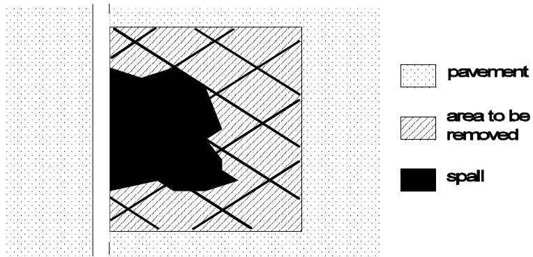
Figure 11. Sawing pattern for large repair areas.
