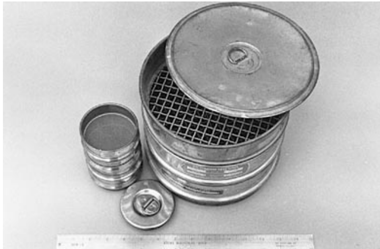
Figure 2-19 SIEVES. Types of sieves used in examination of concrete and concrete materials, 8in. and 3in. sizes.
