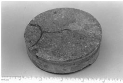
Figure 10-9 ALKALI-SILICA GEL. A. Gel exuding at deteriorating portion of pavement. B. Gel on surface of core removed from deteriorating pavement. Notice the 1200 cracking.
