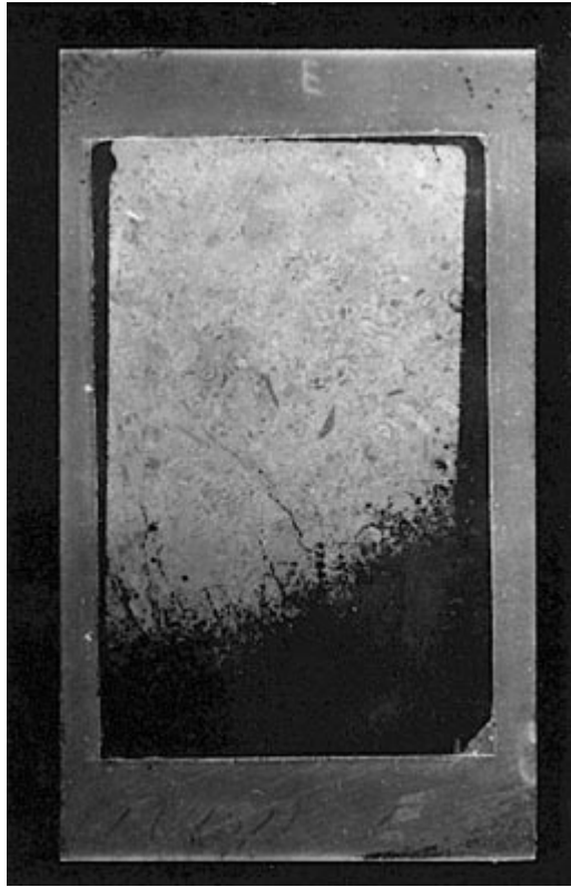
Figure 5-5 THIN SECTION THINNED TO NOTHING ON ONE END.
