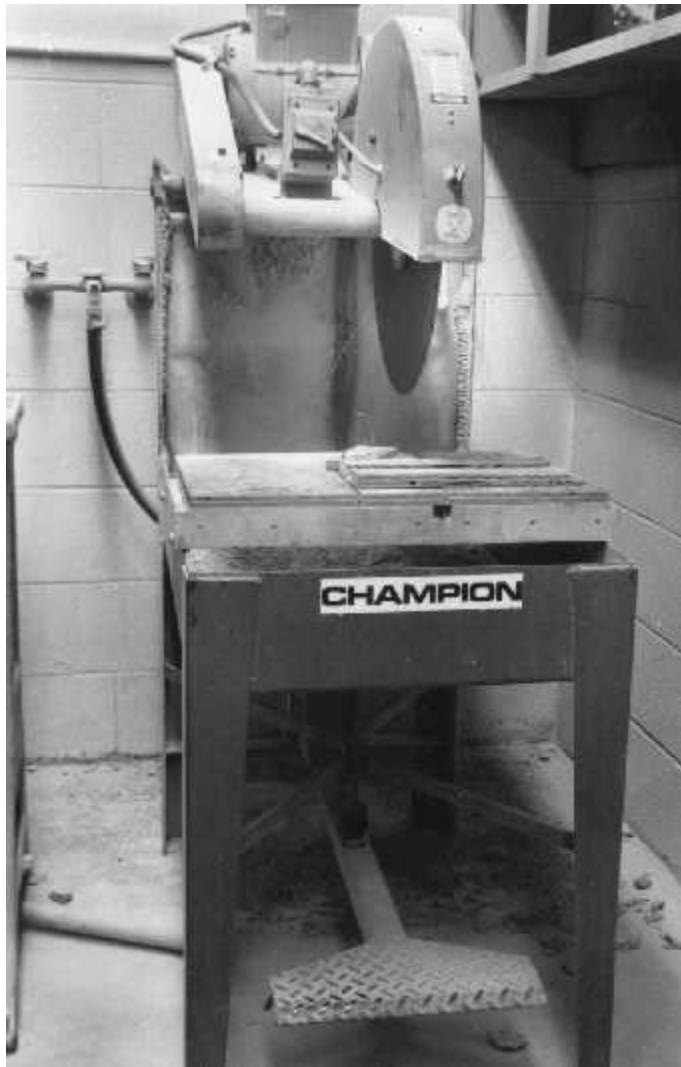
Figure 2-3 WATERCOOLED, DIAMOND-EDGED, ROTARY SAW WITH OVERHAND ARM.
