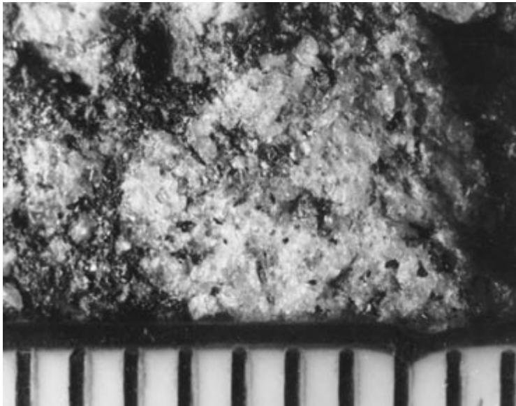
Figure E-5 TRAFFIC-WORN SURFACE OF GRANITE AGGREGATE PARTICLE.
