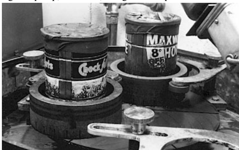
Figure 2-8 WEIGHTS. For lapping slices smoothly.
