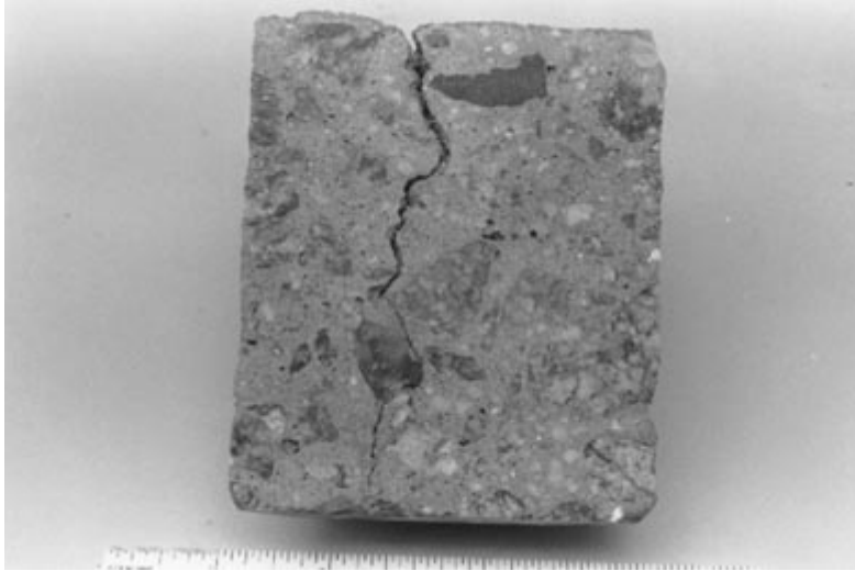
Figure 4-6 PLASTIC SHRINKAGE CRACK. On a lapped surface. The wearing surface is at the top of the photograph.
