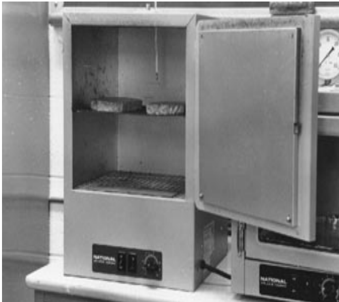
Figure 2-13 DRYING OVEN. Thermostatically controlled.
