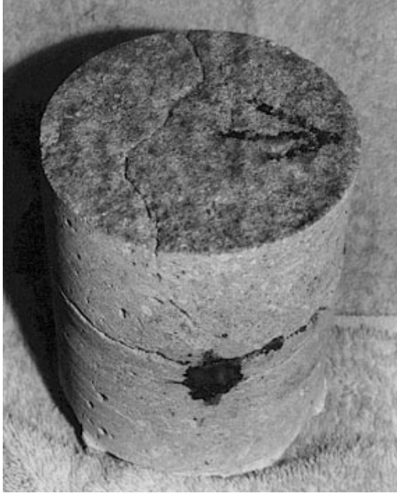
Figure 3-5 CRACKING ON SURFACE AND SIDE OF CORE. With associated corrosion and expansion of the reinforcing bar.
