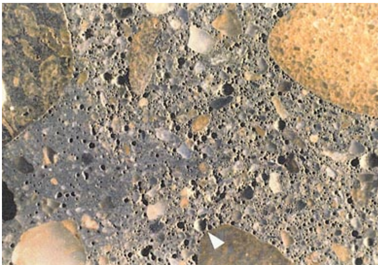
Figure 6-3 SURFACE OF FINELY LAPPED SLICE OF CONCRETE CONTAINING 17% TOTAL AIR VOIDS.
