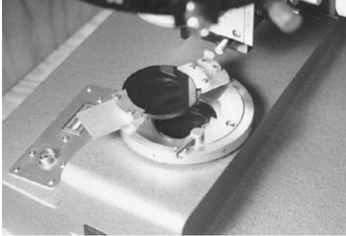
Figure 13-4 SWING-OUT FILTER OVER LIGHT PORT ON BASE OF MICROSCOPE.
