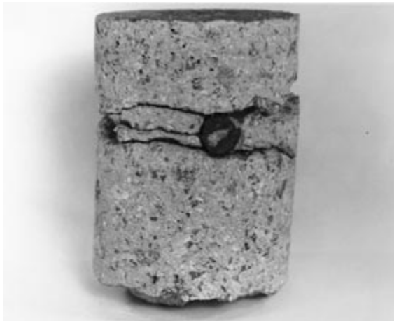
Figure 3-5 CRACKING ON SURFACE AND SIDE OF CORE. With associated corrosion and expansion of the reinforcing bar.
