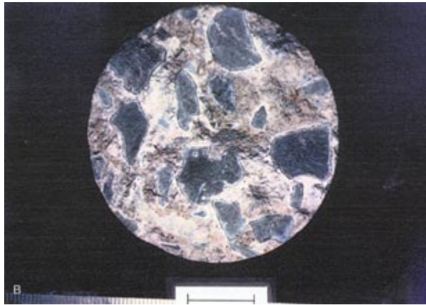
Figure 10-8 ALKALI-SILICA REACTION IN LONGITUDINALLY REINFORCED PAVEMENT CONSTRUCTED WITH DARK METABASALT AGGREGATE.
