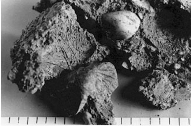
Figure 3-7 FRAGMENTS OF CONCRETE DESTROYED BY FREEZING BEFORE FINAL SETTING. The scale is in intervals of 1/8 in.
