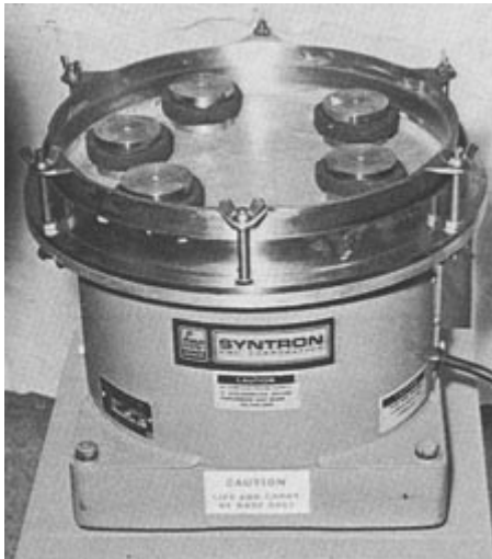
Figure 2-15 MOUNTED SET OF CLAMPS. The little rectangles of lucite are used to distribute stress (Walker & Marshall, 1979).
