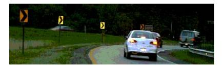
Figure. Post-Mounted Delineators.
