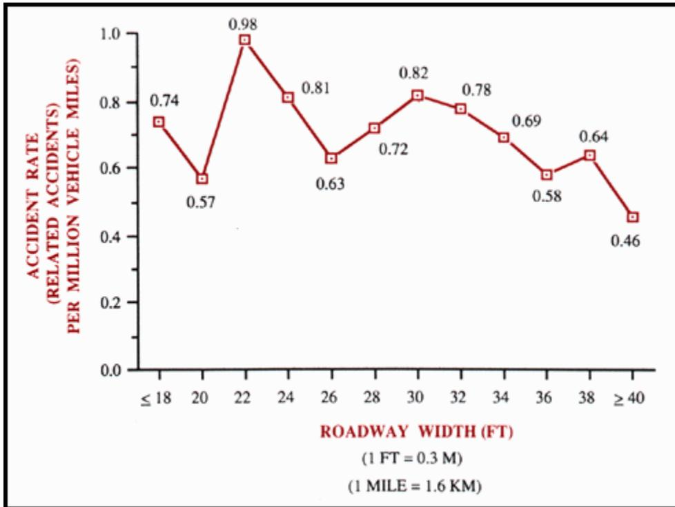
**Figure 2. Relationship between accident rate and total width for unpaved roads in Minnesota.**
