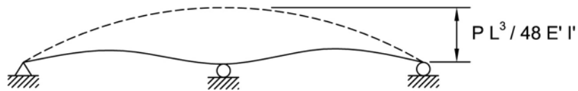
(c) Restoration of redundant support.
