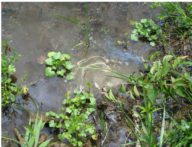
Figure A2-17 Sand boil documented during field reconnaissance during high water event.
