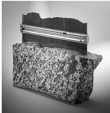
Figure 9-22 Profile gauge for measuring discontinuity roughness (courtesy of Controls Group).
