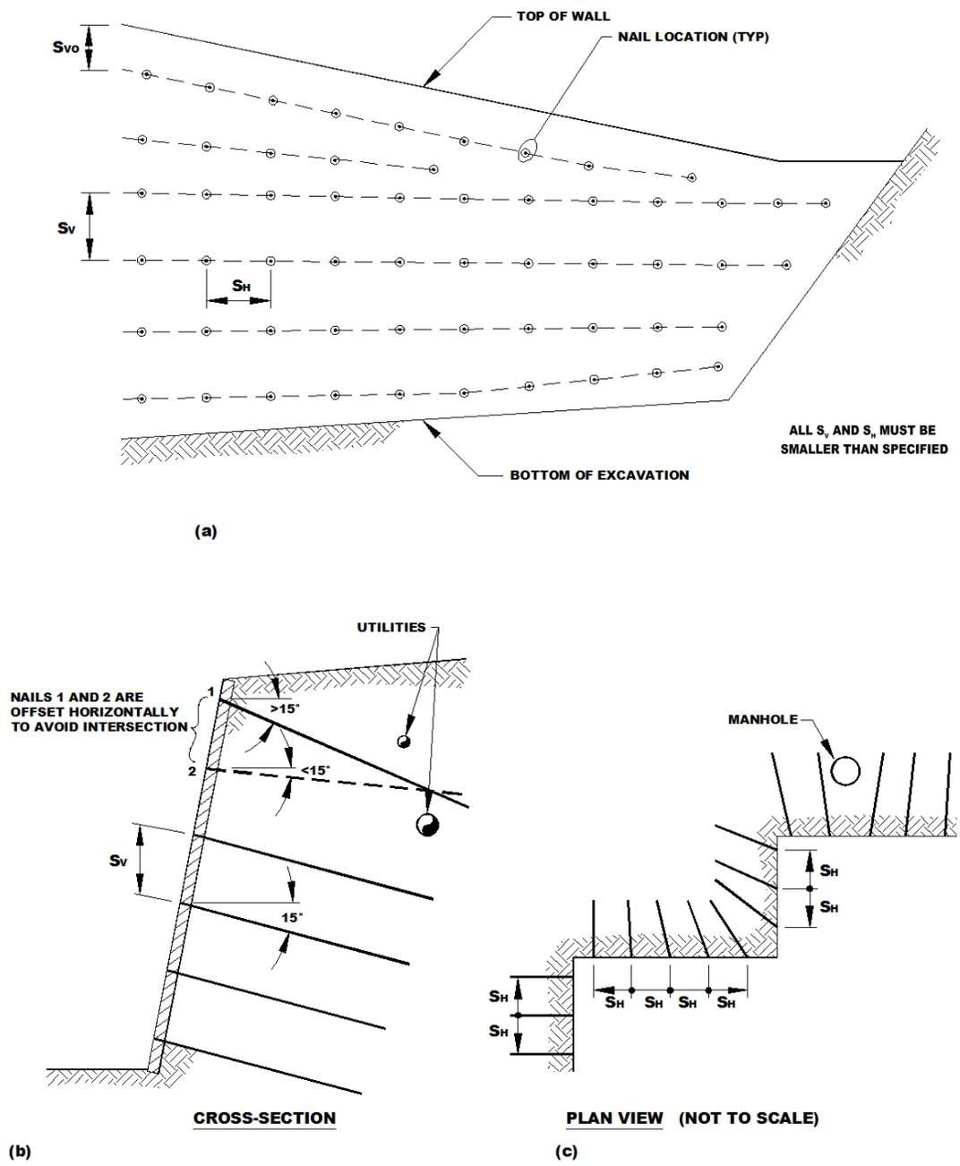
Figure 6.2: Illustration. Varying nail patterns: (a) example of nail arrangement for non-horizontal ground, (b) varying nail inclination and lengths around utilities, and (c) nail splaying at corners.
