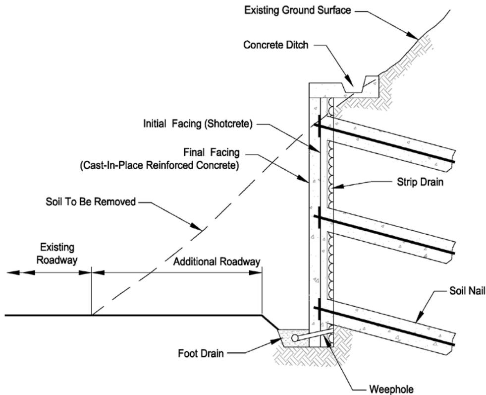
Figure 2.4: Illustration. Roadway cut supported with soil nails. Modified after Porterfield et al. (1994).
