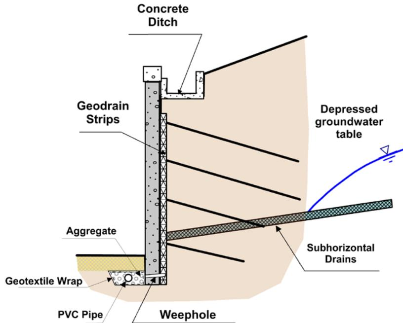
Figure 6.12: Illustration. Drainage of soil nail walls.
