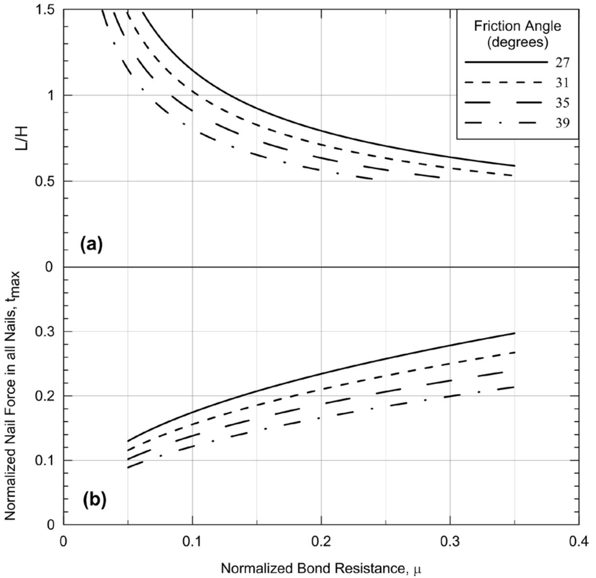
Figure B.2: Chart. Batter = 0 deg. - Backslope 0 deg.
