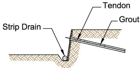
**Step 3. Install and Grout Nail**
