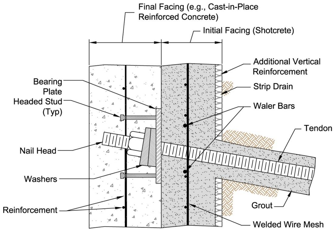
Figure 2.1: Typical cross-section of a soil nail wall. Modified after Porterfield et al. (1994).
