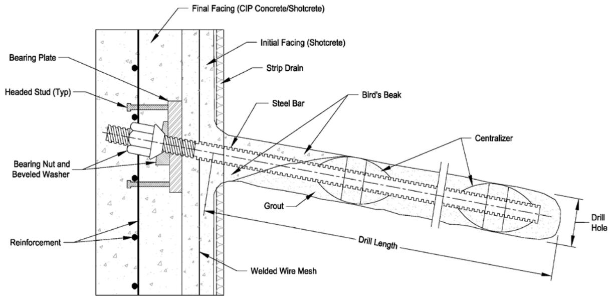
Figure 3.1: Illustration. Main components of a solid bar soil nail and associated wall facing. Modified after Porterfield et al. (1994).
