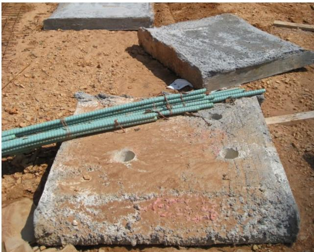
Figure 3.11: Photo. Shotcrete test panel cored for compressive testing of recovered
