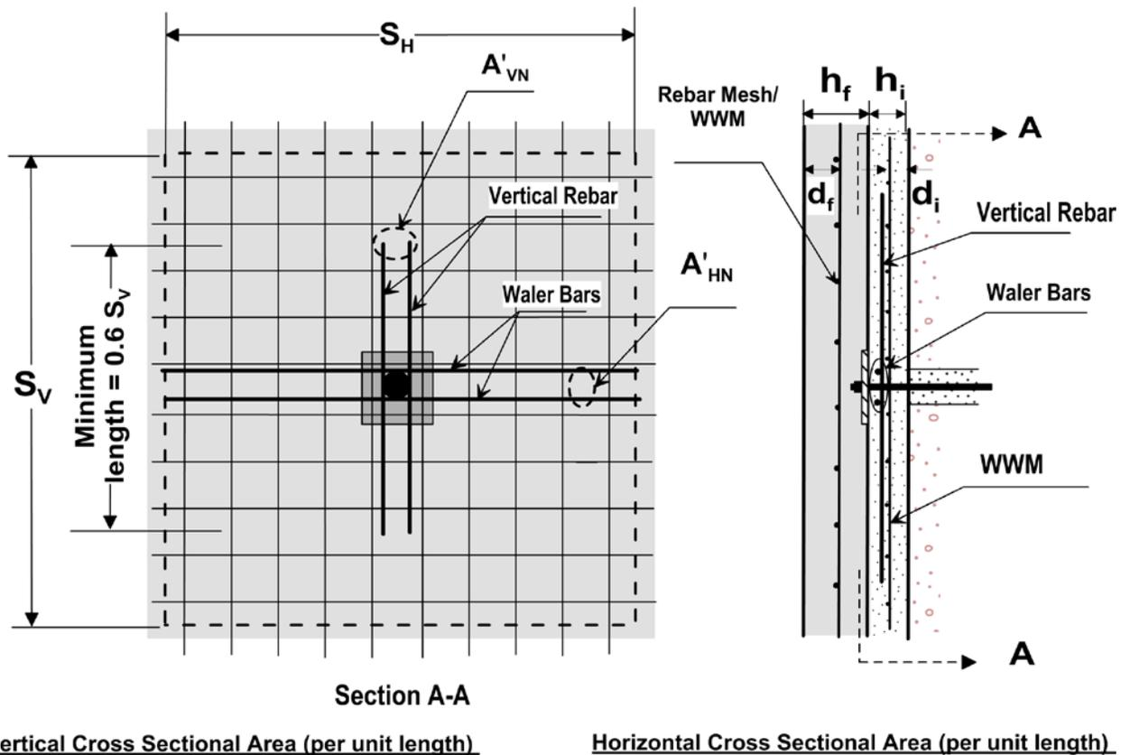
Figure 6.5: Illustration. Reinforcement nomenclature for facing in bending.
