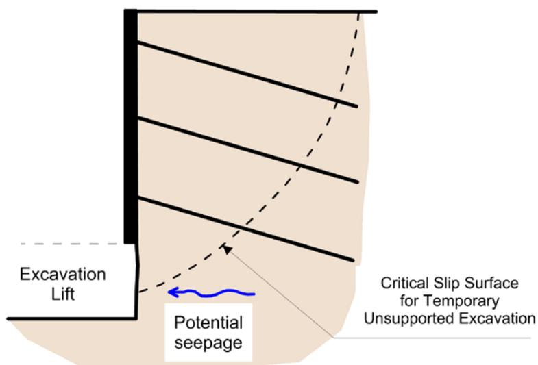
Figure 5.2: Illustration. Potential critical stability case during construction.
