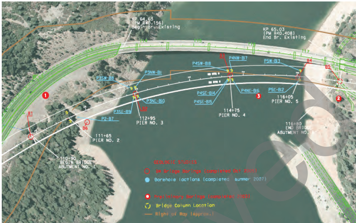
Figure 2-10 Example of Site Investigation Plan Location Map, Sacramento River Bridge Replacement (Courtesy of Caltrans)
