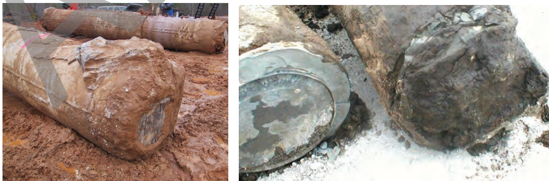
Figure 4-23 Exhumed Shafts after Grouting
