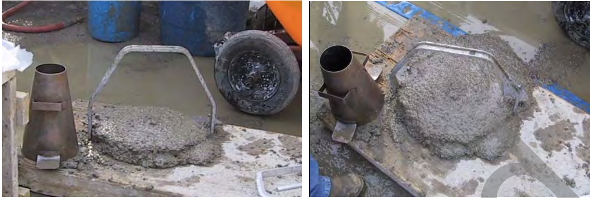
Figure 9-25 Concrete with High Workability but with Potential for Bleeding and Segregation
