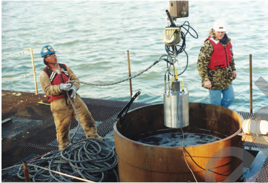
Figure 19-2 Shaft Inspection Device for Visual Inspection of the Shaft Bottom in a Wet Excavation (60-inch diameter shaft shown).
