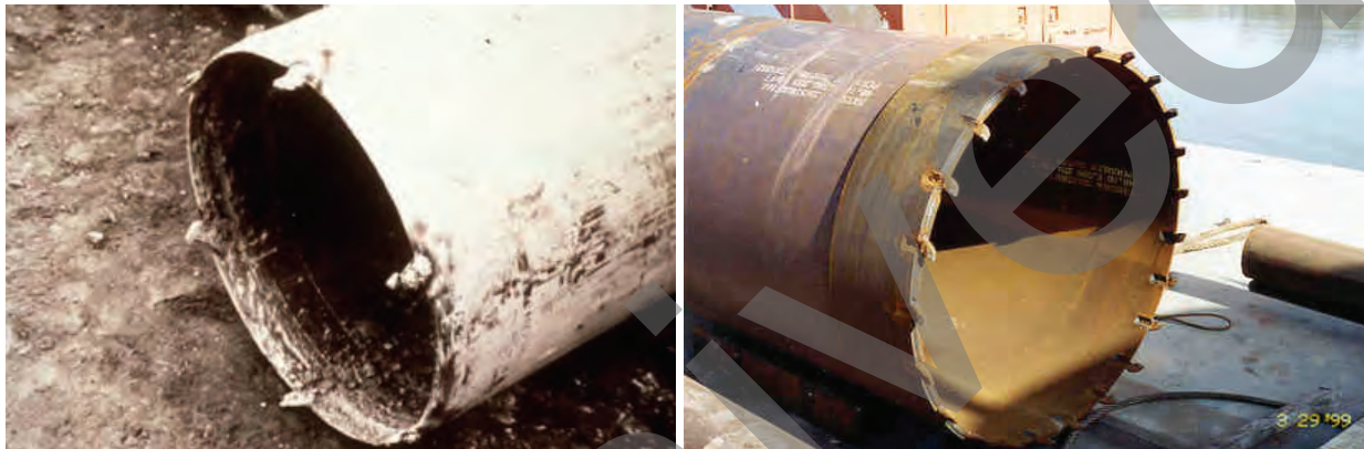
Figure 6-6 Teeth for Use in Sealing Casing into Rock (Photograph at top left courtesy of Herzog Foundation Drilling, Inc.)
