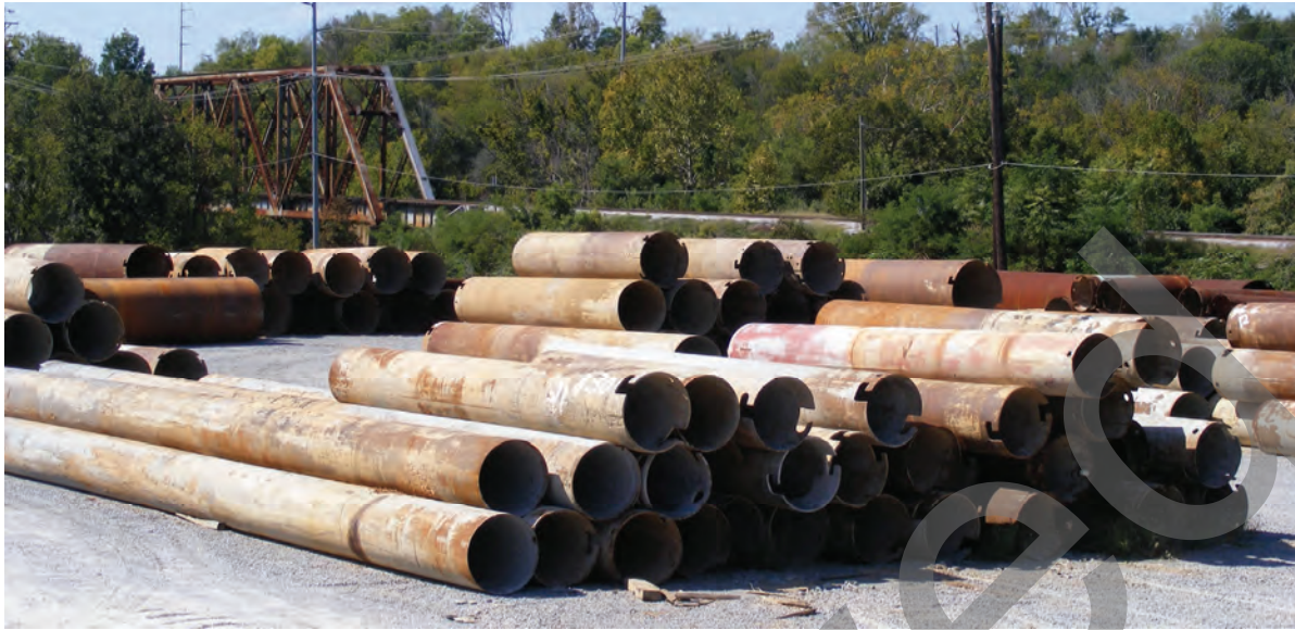
Figure 6-1 A Typical View of Stored Temporary Casing
