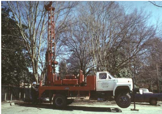
Figure 3-25. Views of Rotary Drill Rigs Mounted on Trucks for Soil & Rock Exploration.
