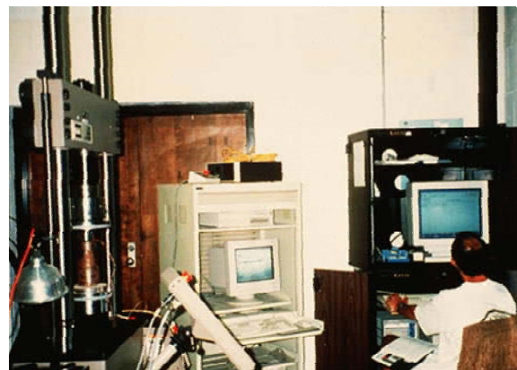
Figure 8-1: (a) Intact Rock Specimens for Laboratory Testing; (b) Compressive Strength Testing.
