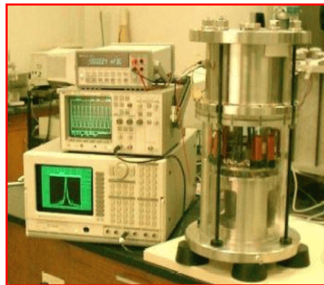
Figure 7-12. Resonant Column Test (RCT) Equipment for Determining G_{max} and D in Soils.
