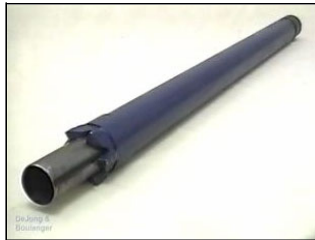
Figure 3-14. Pitcher Tube Sampler.
