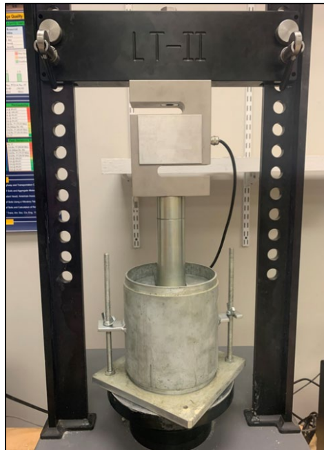
Figure 20. Photo. Test setup for CBR test.
