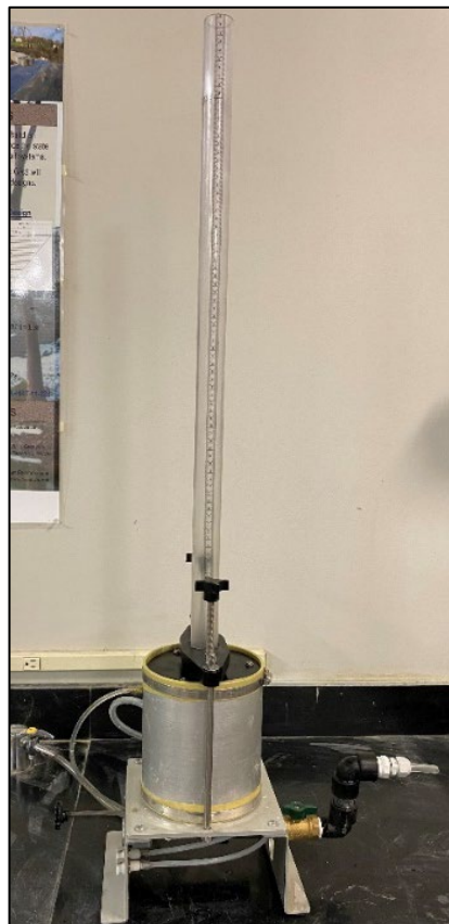
Figure 15. Photo. CTB FH permeability test setup.
