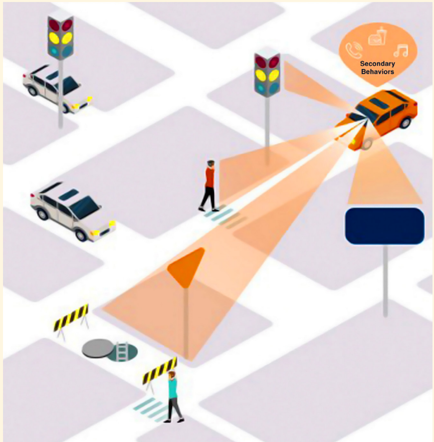
© Virginia Tech Transportation Institute. Computer vision can annotate secondary behaviors inside the vehicle, extravehicular context, and interactions between the driver and the environment. (6)
