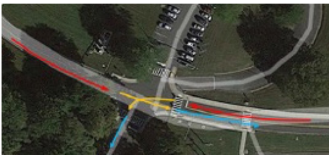
Source: FHWA. Transportation systems management and operations testing scenarios. The arrows show the intended path of travel for each vehicle optimizing its approach to the intersection. (11)
