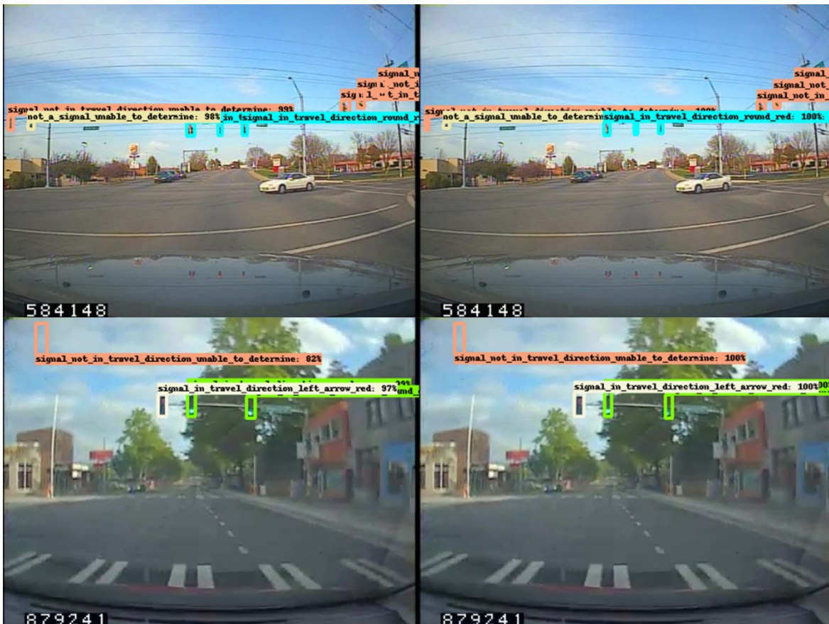
© Volpe National Transportation Systems Center. Researchers are training neural networks to detect traffic signals and signal states. (6)
