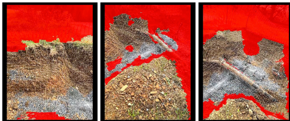
Figure 4. Screenshots. Data collection session with 3D Scanner App where areas beyond the sensor range are masked.
