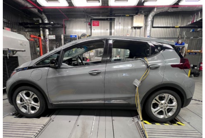
Figure 3. Image. Example of a vehicle-in-the-loop simulation.
