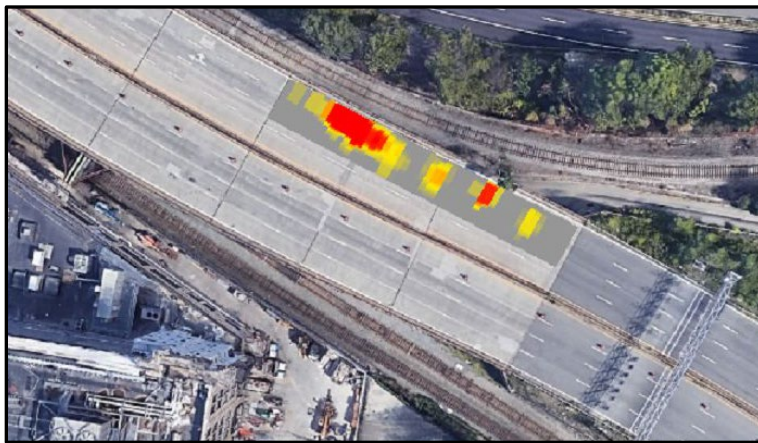
Figure 21. Photo. IE findings on spans 1 through 3 of a bridge deck (Google® Earth 2020).
