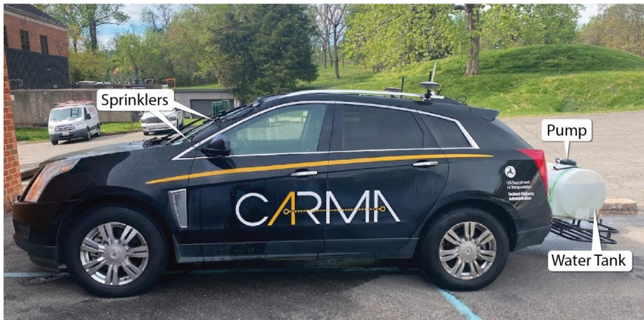
Figure 1. Photo. Sprinkler system used to simulate rainfall.
