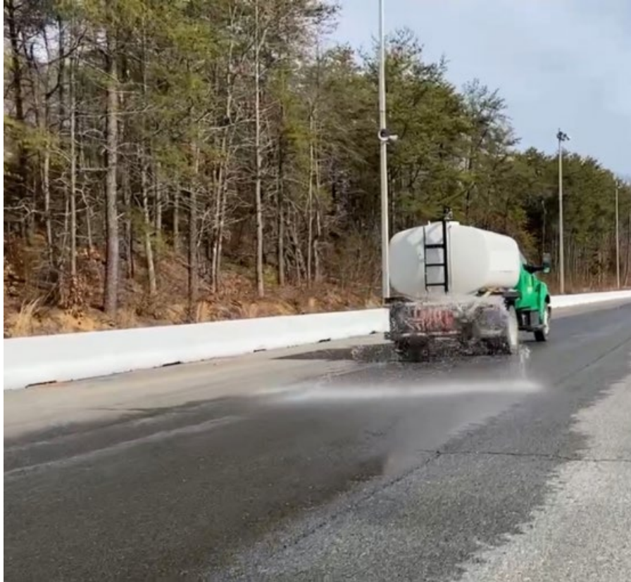
Figure 2. Photo. Wet pavement simulation.
