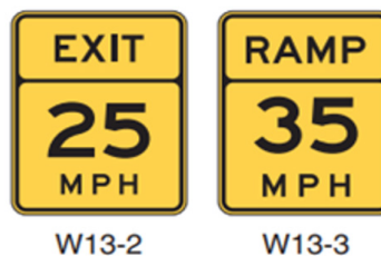
Figure 1. Illustration. Advisory Exit and Ramp Speed signs (FHWA 2009).
