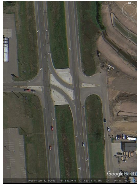
Figure 20. Photo. MN-65 at 187th Lane intersection, overview of main intersection and U-turns, after condition in East Bethel, MN. (32)
