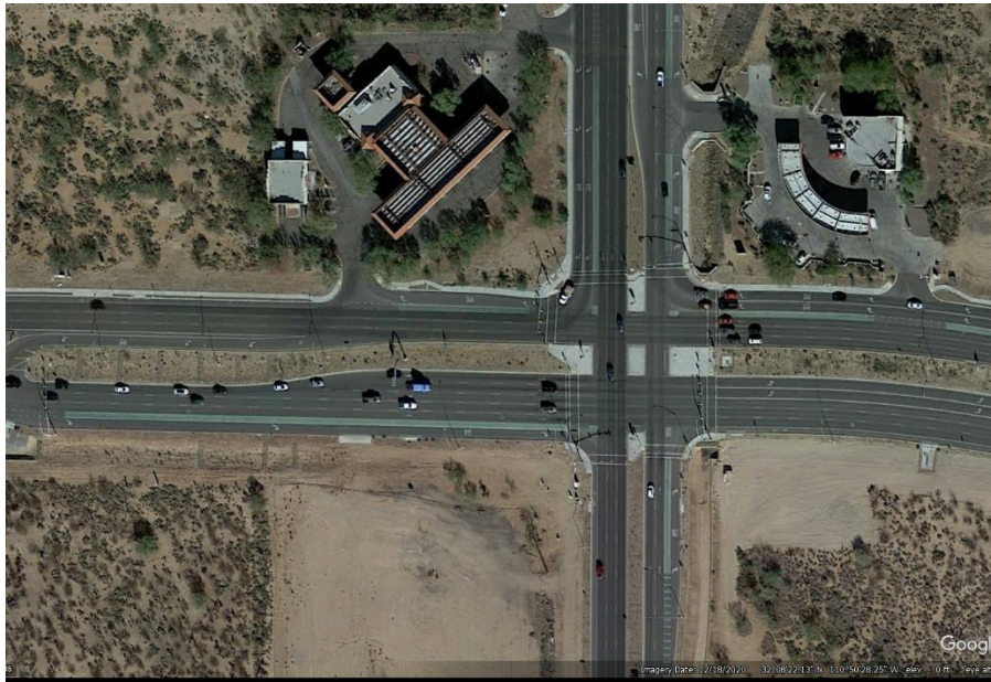
Figure 11. Photo. Valencia Road at Kolb Road intersection, overview of main intersection and U-turns, after condition in Tucson, AZ. (32)
