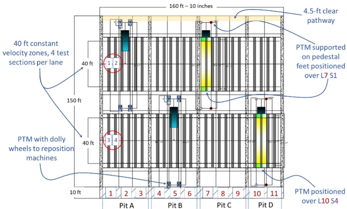
Figure 12. Illustration. Third-generation pavement test pits.
