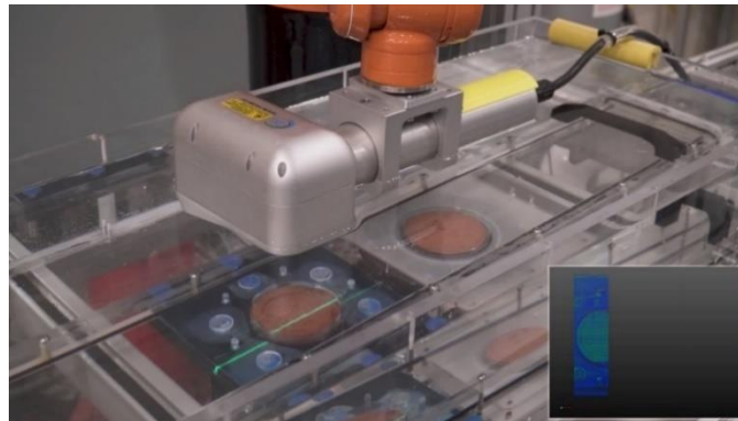
Figure 20. Photo. Laser scan of soil surface and digitized soil surface (inset).
