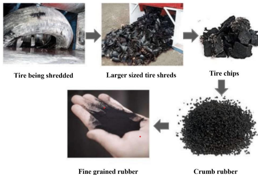
Figure 22. Illustration. Rubber shredding procedure and outputs (Creative Commons n.d.c).
