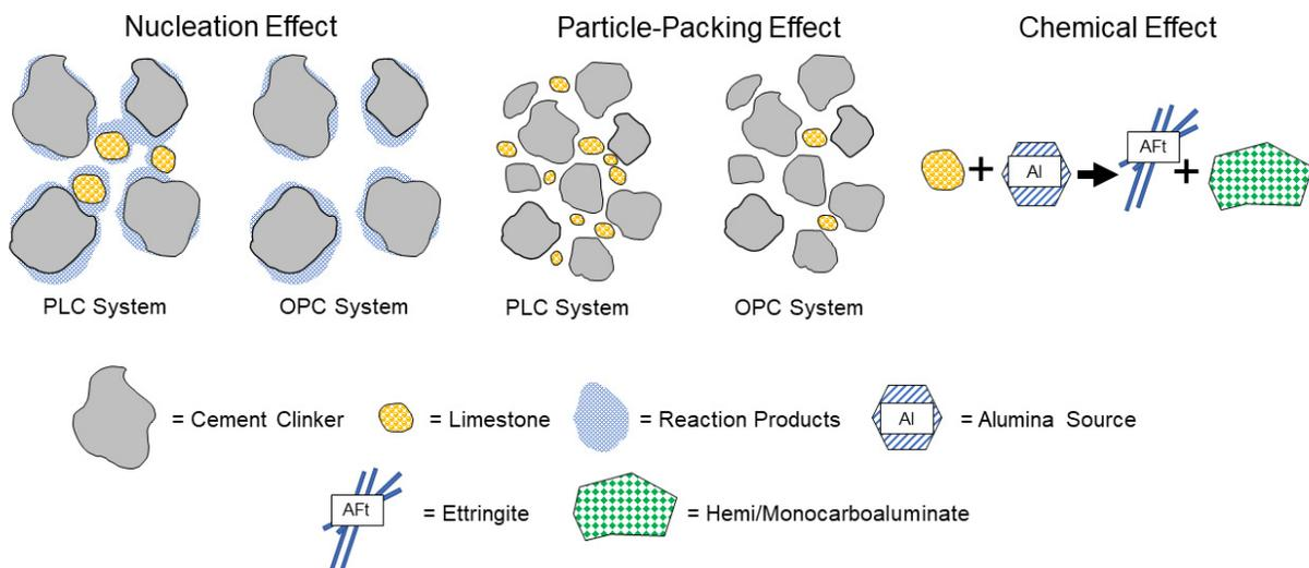
with traditional, OPC-SCM systems.<sup>(31)</sup> This increase in pozzolanic reactions can potentially contribute to reductions in pore connectivity and thus result in improved concrete transport properties (e.g., rapid chloride permeability test (RCPT) or resistivity) of concrete.<sup>(31)</sup>
