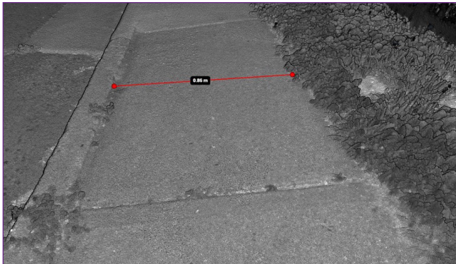
© 2022 Marshall & Coppola. Figure 2. Image. Sidewalk width captured from LiDAR point cloud data. (1)
