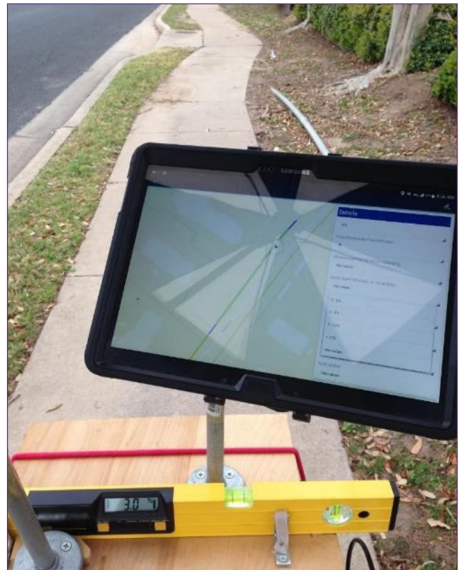
© 2022 City of Austin. Figure 5. Image. City of Austin, TX, sidewalk condition data collection. (1)
