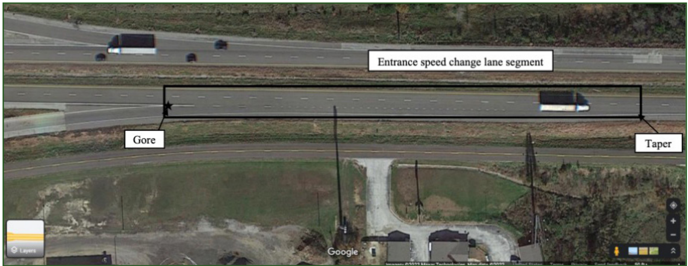
Original photo: Imagery © 2020 Maxar Technologies. Map data © 2020 Google®. Modifications by FHWA (see Acknowledgments section). Figure 2. Map. Real-world example of an entrance speed change lane.
