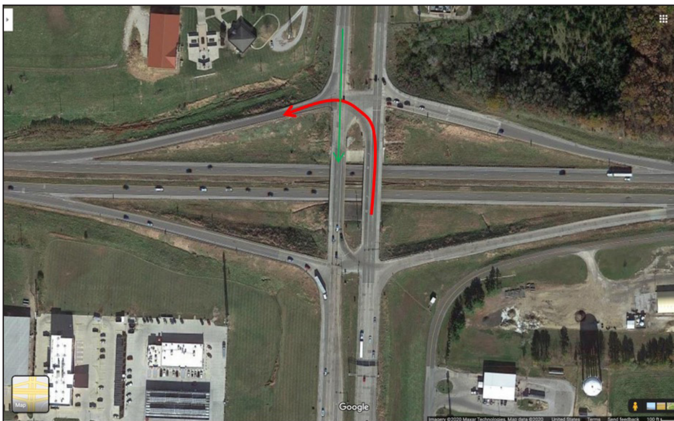
Original photo: Imagery © 2020 Maxar Technologies. Map data © 2020 Google®. Modifications by FHWA (see Acknowledgments section). Figure 1. Map. Example of a diamond interchange with two ramp terminals.
