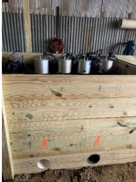
Figure 24. Photo. HVSR four-sensor test setup for soil box 1, lift 4.
