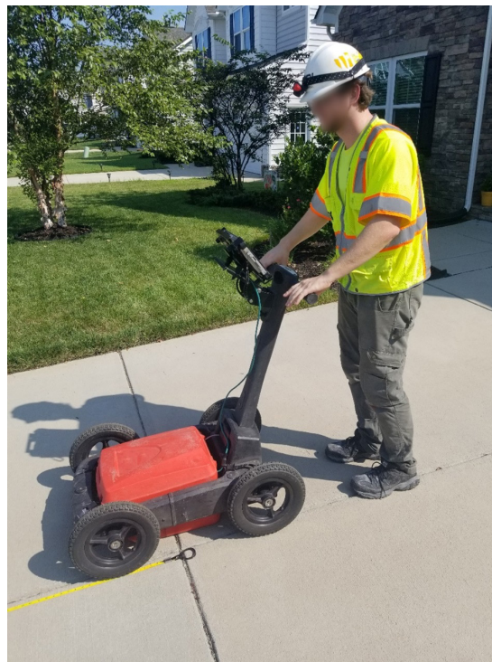
Figure 29. Photo. GPR system with DF antenna.
