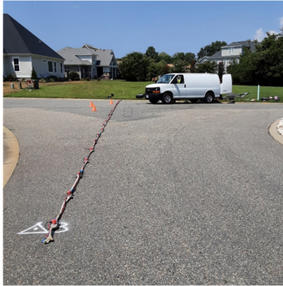
Figure 33. Photo. MASW data collection using a streamer geophone array at Settlers Ridge setup 9, deployed on asphalt.
