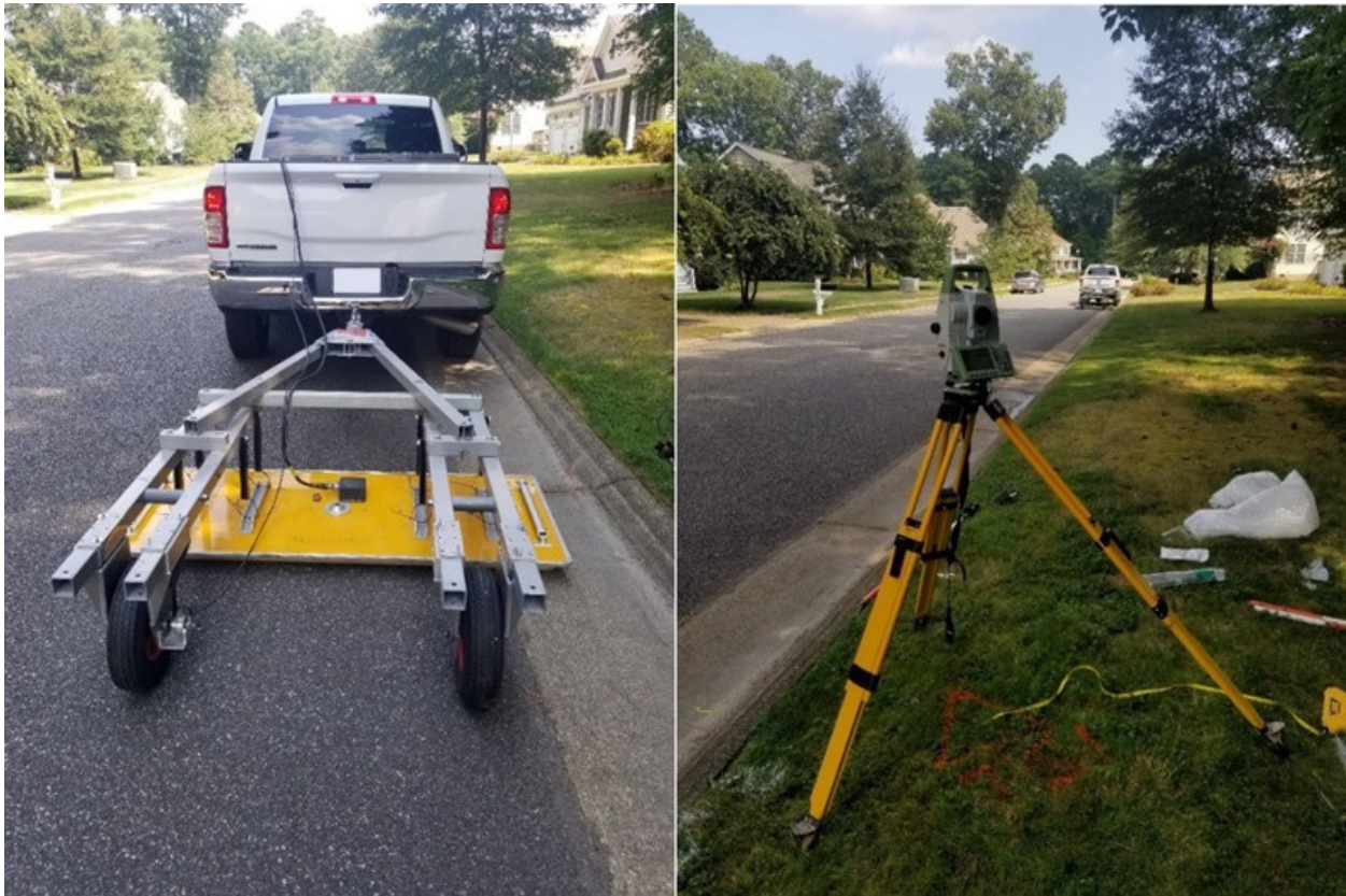
Figure 30. Photos. Photo on left shows a stepped-frequency GPR system mounted on a travel vehicle, and photo on right shows a total station surveying system used to track the GPR antenna positions.
