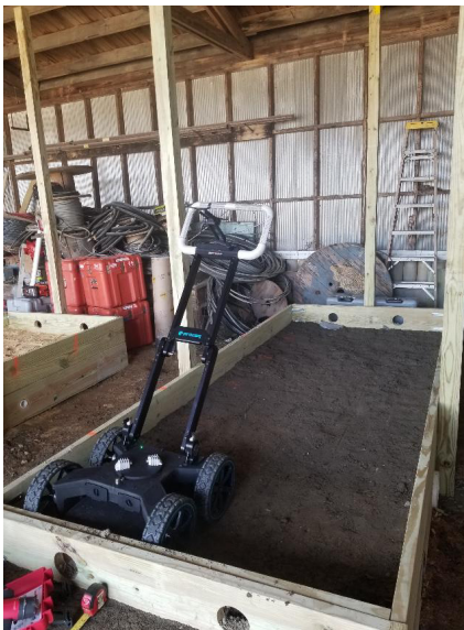
Figure 15. Photo. GPR system with integrated cart scanning soil box.
