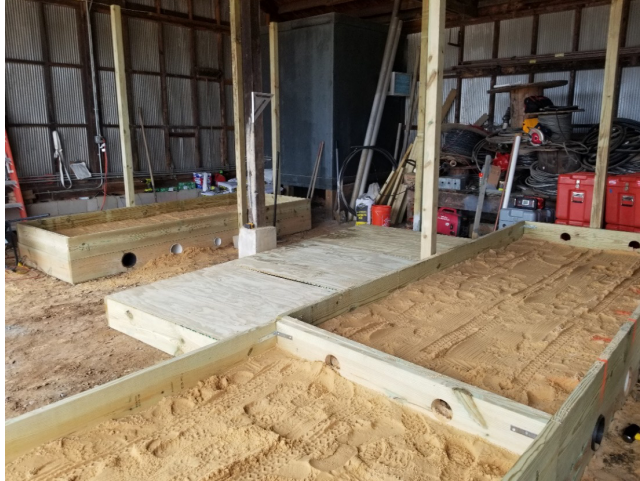
Figure 14. Photo. First level of soil box specimens with buried utilities in parallel.
