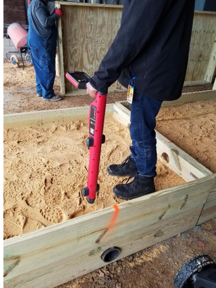
Figure 20. Photo. Underground utilities locator scanning over steel pipe.
