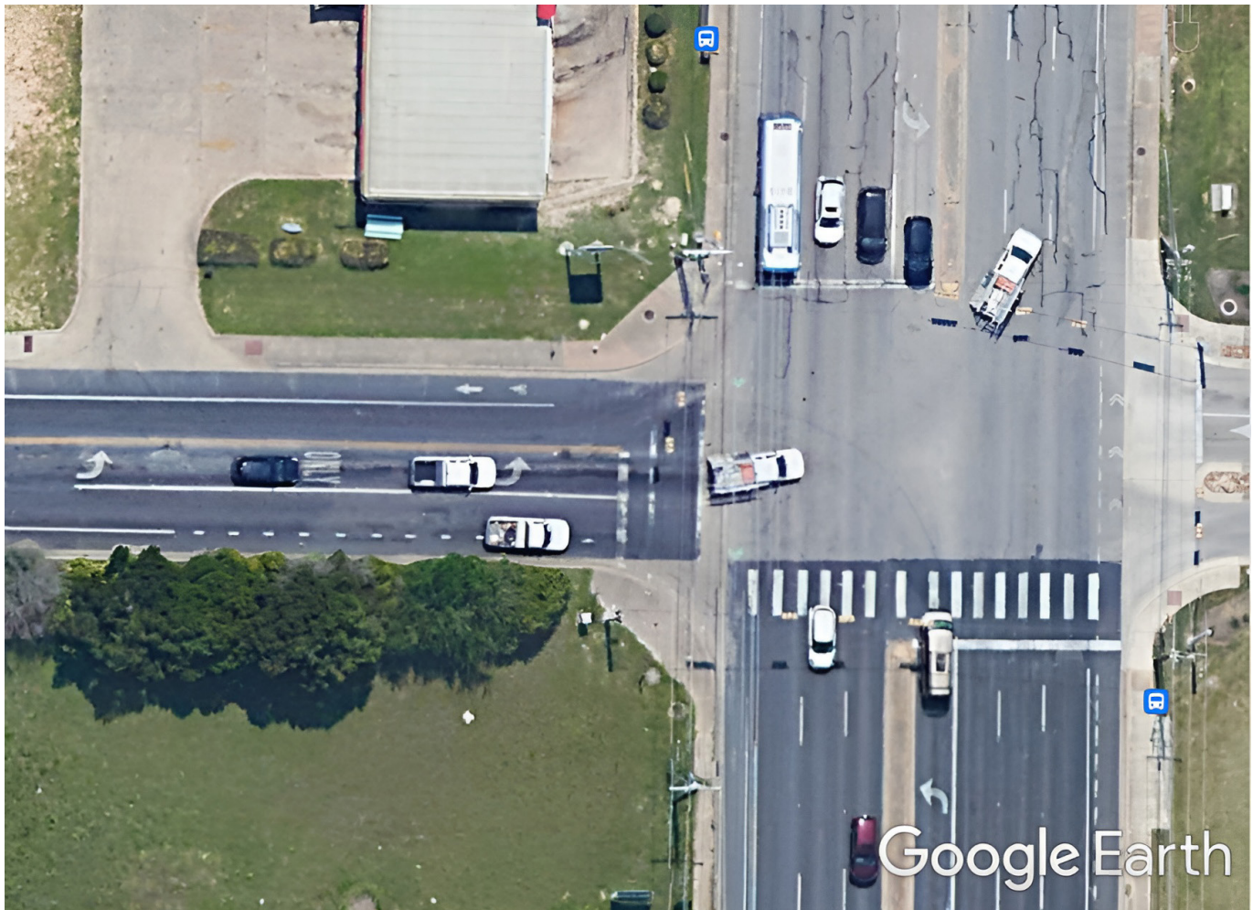
Figure 1. Map. Sample intersection with mixing zone for a bicycle lane, multivehicle through lane, and right-turn movements.
