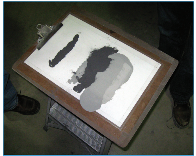
A clipboard showing samples of fly ash before and after electrostatic separation to reduce the amount of carbon in fly ash. Source: FHWA.
