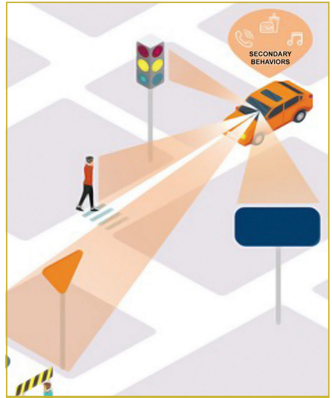
Computer vision can annotate secondary behaviors inside the vehicle, extravehicular context, and interactions between the driver and the environment. © Virginia Tech Transportation Institute.
